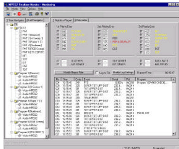
Bild 1.10 MPEG2 REAL TIME MONITOR: Tree Navigator, Statistics und Report
