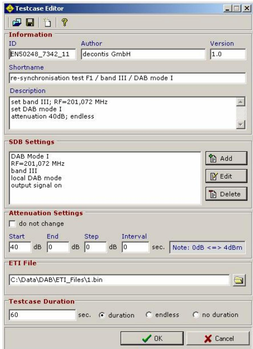
Fig. 3-1: DAB Test Client – Testcase Editor
