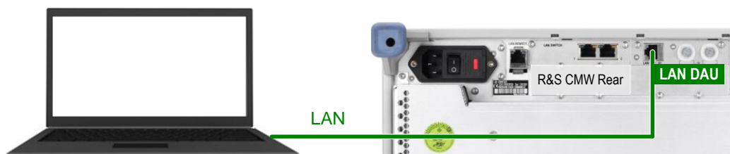
Fig. 3-4: End-to-end test setup with LAN-connected PC
