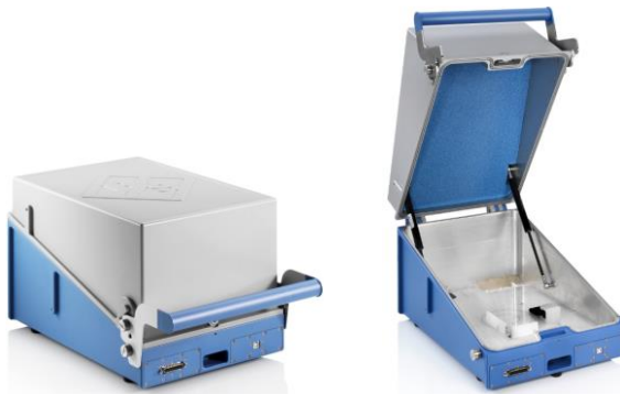
Fig. 3-2: R&S®CMW-Z10 RF shielding box
