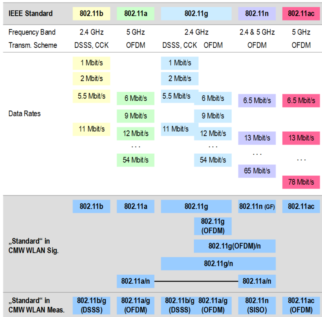
Fig. 2-1: WLAN standards, data rates (20 MHz channels) and mapping on the CMW “Standard”
