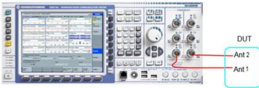
c: Connecting the CMW500 to a CA DUT with a dual-antenna design
