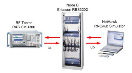
Before the R&S CMU300 can test the RF parameters according to [1], the Node B must be altered to a test mode with the above-mentioned test scenarios. In most cases these test modes are not supported by the radio network controller (RNC) of the operative network. In this particular case the NH RNC/lub Simulator assumes this role. The BTS, being isolated from the network, is activated by the NH RNC/lub Simulator via the lub interface. The BTS is then tested as follows:
