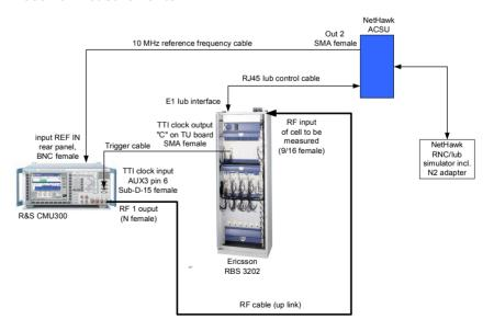
**Note:** If the BTS uses remote amplifiers (tower-mounted), these must be taken into consideration in the test setup, that is, the R&S CMU300 must be directly connected to the RF connectors on the amplifier.
