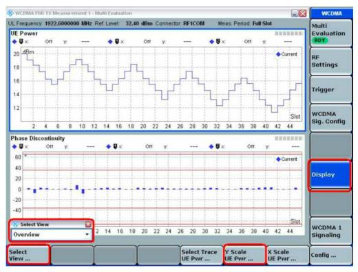
Fig. 30: Configuring the display mode for phase discontinuity.
