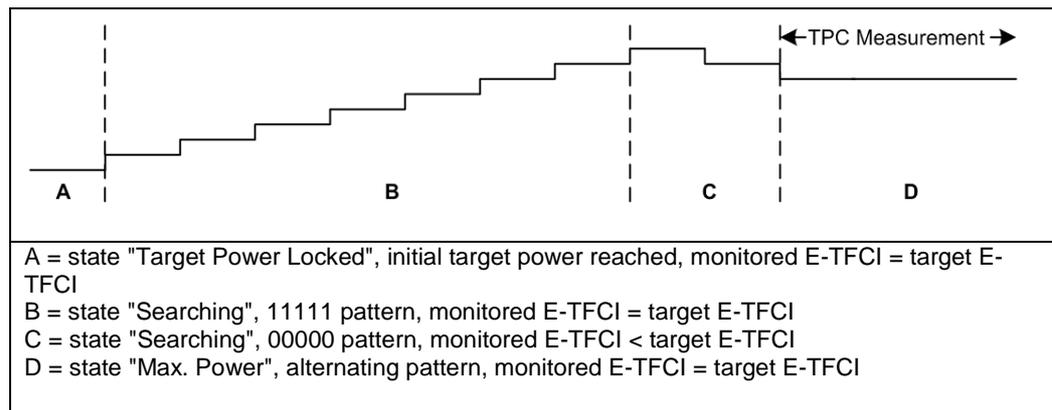
**Figure 13: Arriving at the max. power condition for Subtests 1 through 4.**
