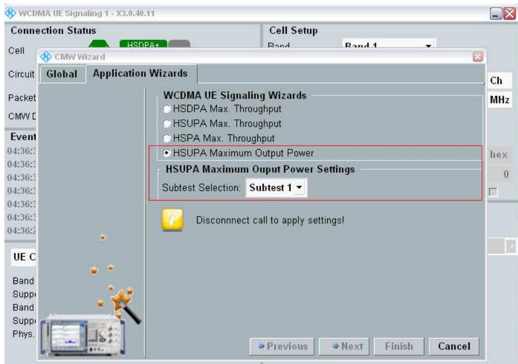
Figure 1: Activating the WCDMA-UE signaling application.
