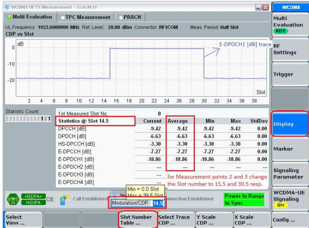
Figure 22: UE relative code domain power accuracy for HS-DPCCH and E-DCH measurement results.
