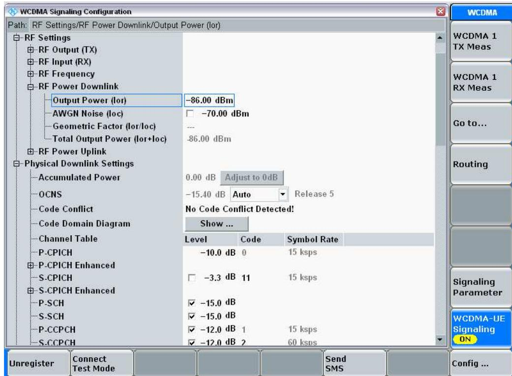
Figure 9: Downlink physical channel configuration in line with Table 16.
