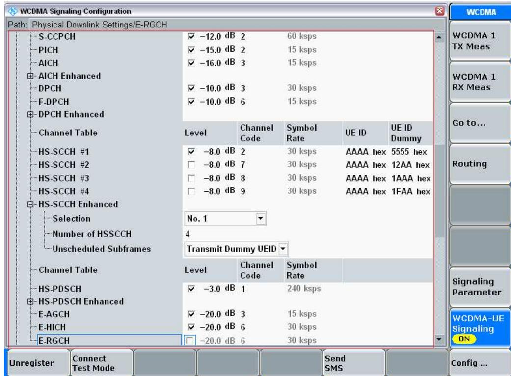
Figure 10: Downlink physical channel configuration in line with Table 16.
