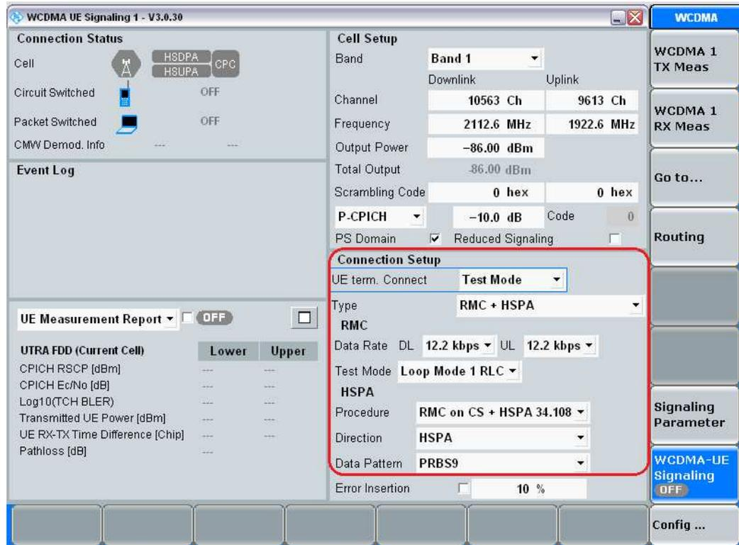
Figure 2: RMC 12.2kbps + HSDPA 34.108 configuration.
