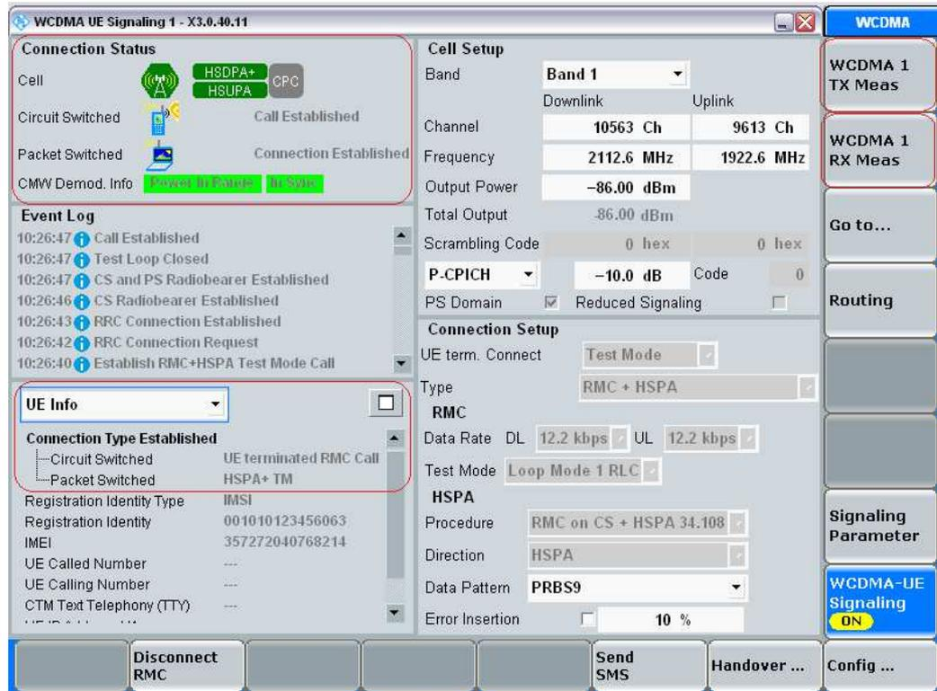
Figure 12: RMC 12.2 kbps + HSPA 34.108 call setup procedure for Subtests 1 through 4.
