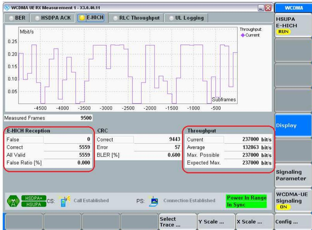
Figure 30: Measurement results for detection of E-HICH (2 ms case).
