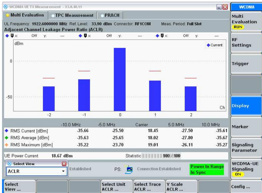
Figure 24: ACLR with E-DCH measurement results.
