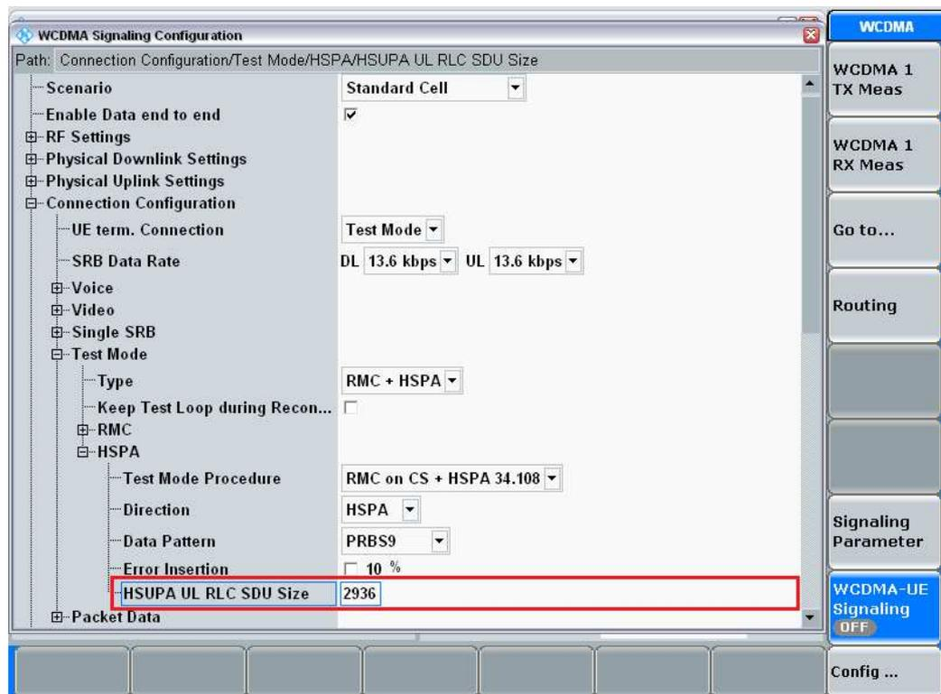
Figure 3: RLC SDU size configuration.
