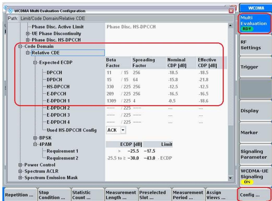
Figure 25: Expected ECDP displayed on the R&S<sup>®</sup>CMW500.
