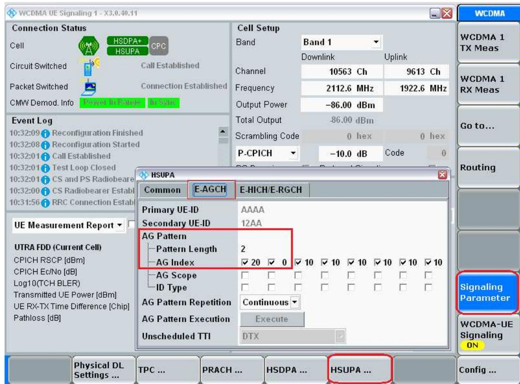
Figure 20: Alternating pattern of absolute grant allocation to the UE.
