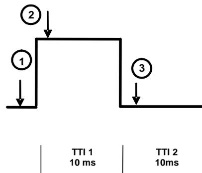
Figure 18: Transmit power profile for UE CDP accuracy.
