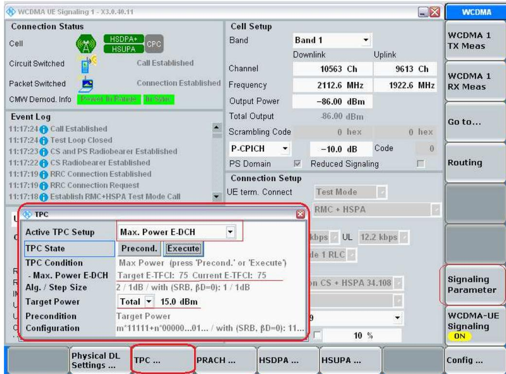
Figure 15: TPC pattern for the Max. Power condition.
