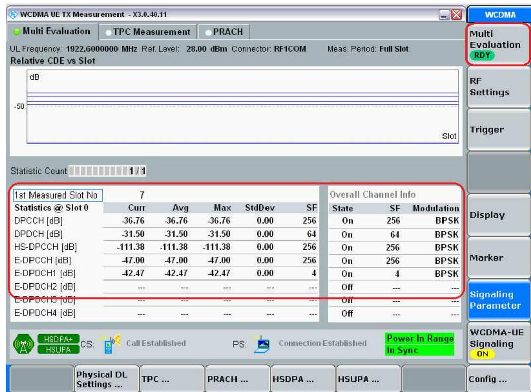
Figure 26: Measurement results for the relative code domain error with HS-DPCCH and E-DCH.
