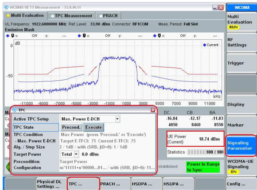
Figure 23: Measurement results for the spectrum emission mask.
