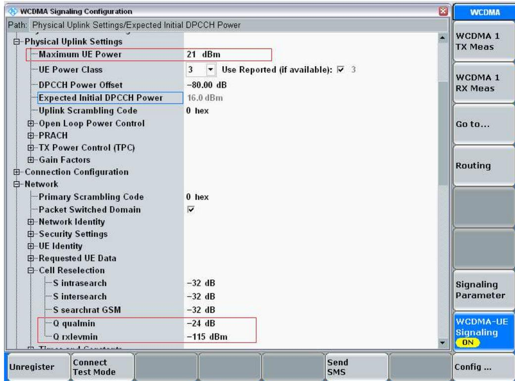
Figure 8: Serving cell parameters.
