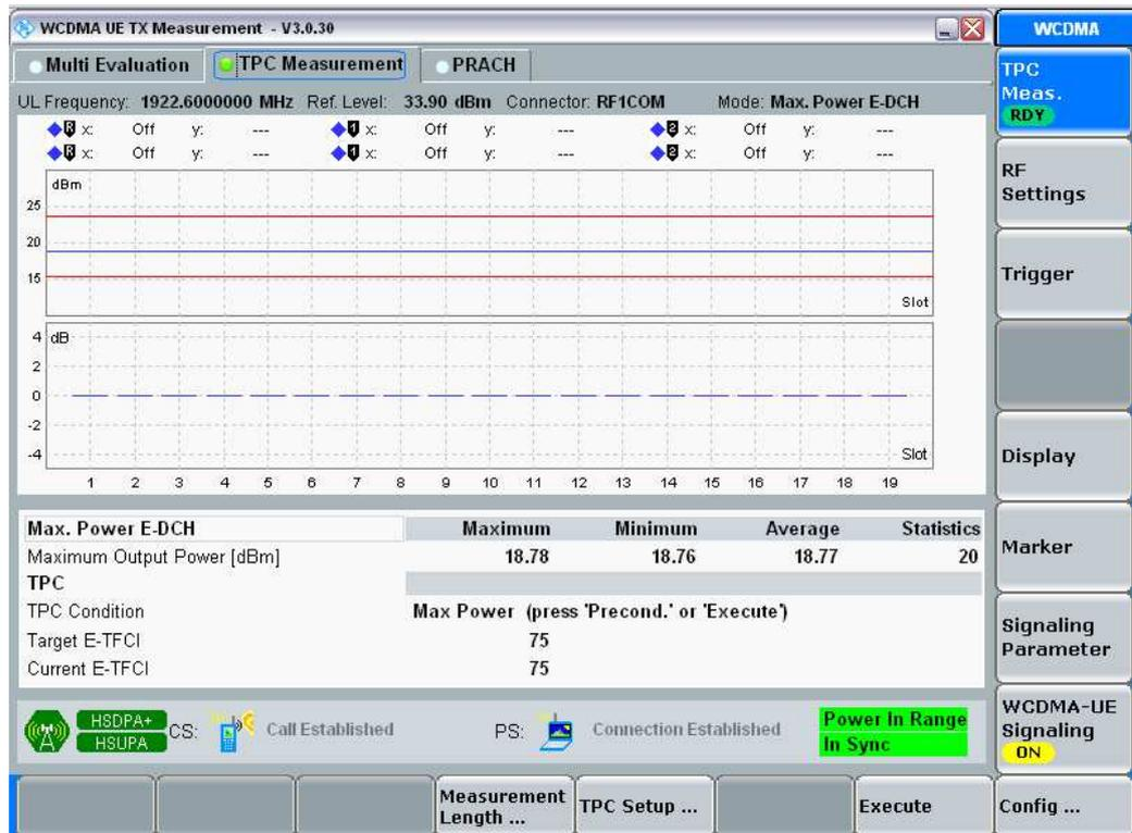
Figure 16: Measurement results for Maximum Output Power with HS-DPCCH and E-DCH.
