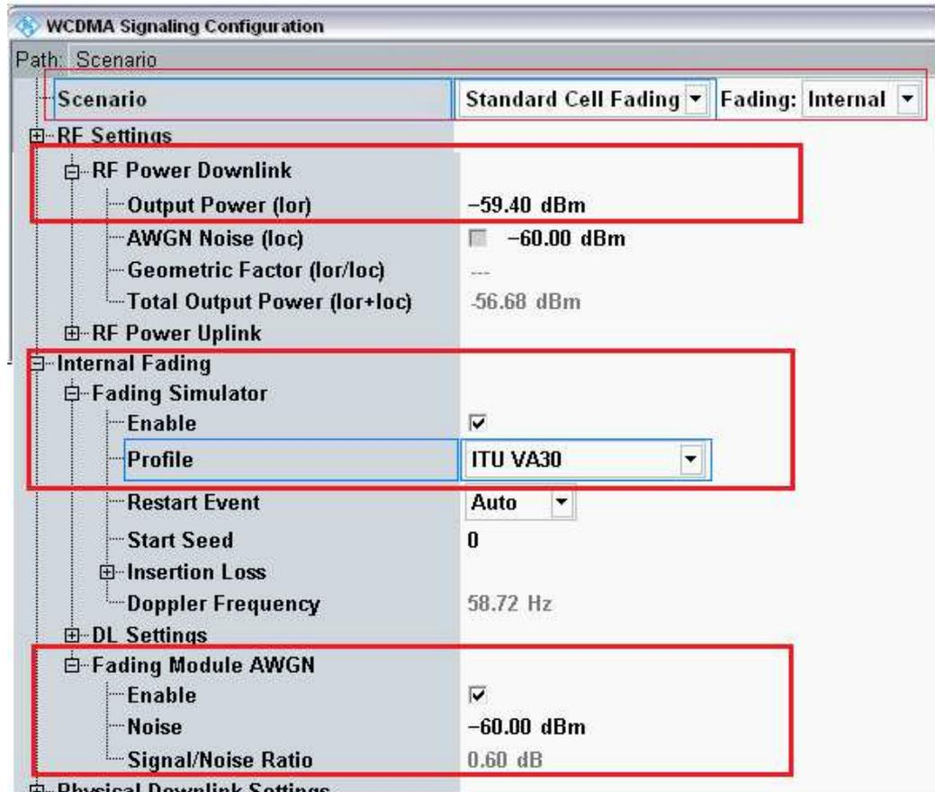
Figure 27: Internal fading simulator on the R&S®CMW500.
