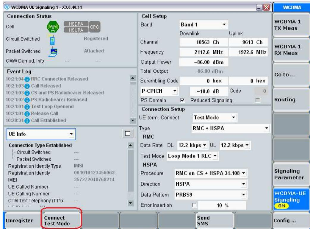
Figure 11: RMC 12.2 kbps + HSPA 34.108 call setup procedure for Subtests 1 through 4.
