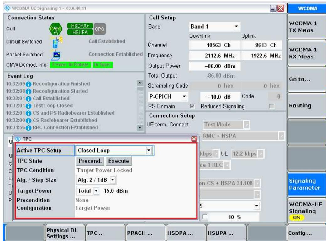
Figure 19: TPC setup to stimulate a UE transmitting at 15dBm  $\pm$ 2dB.
