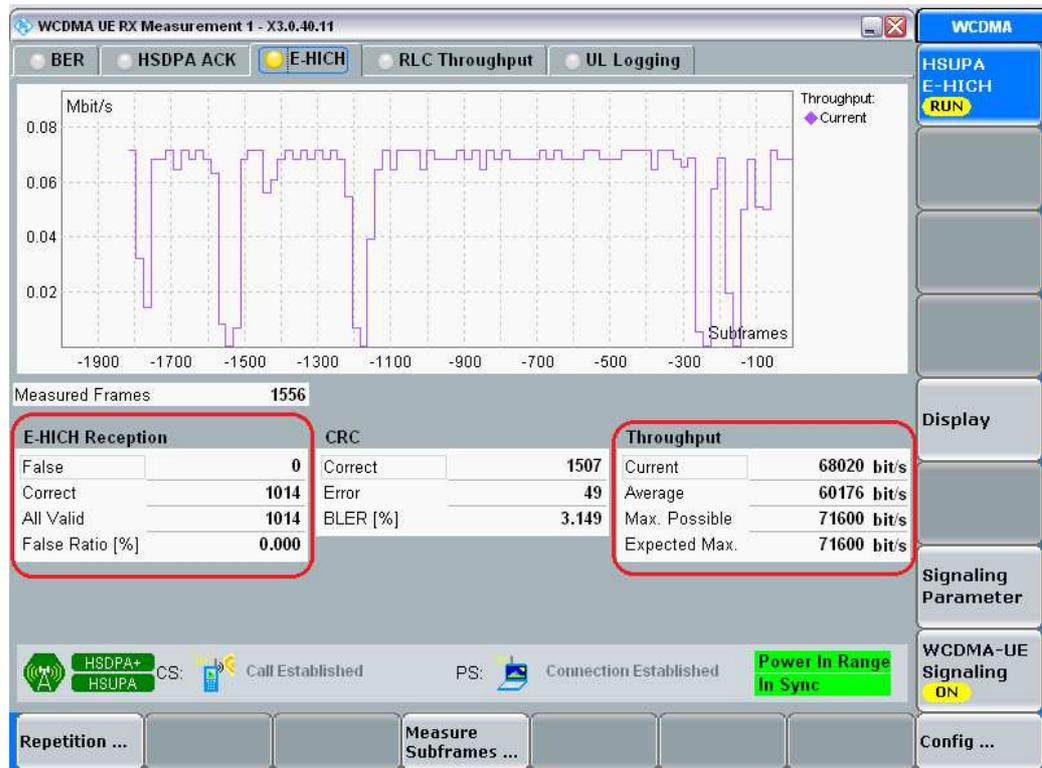
Figure 29: Measurement results for detection of the E-DCH HARQ indicator channel (E-HICH).
