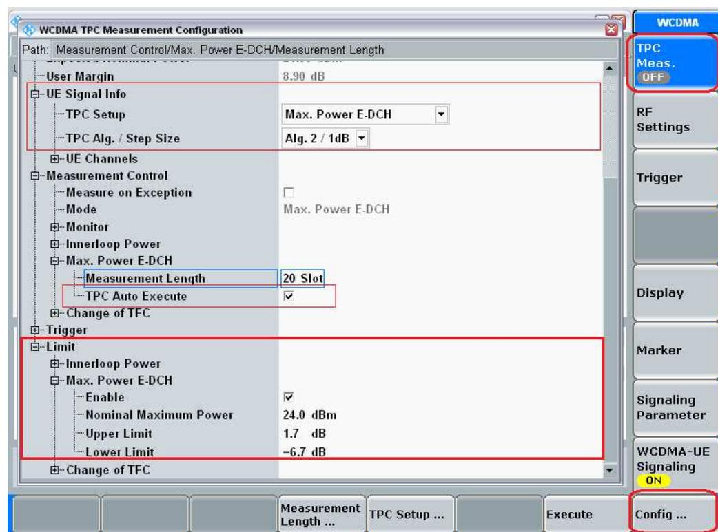
Figure 17: Configuration of limit lines in line with Table 17.
