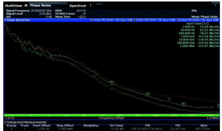
Figure 6: Phase noise measurement at 25.8 GHz (green) with x-corr and at 51.2 GHz without x-corr (orange) and 51.2 GHz with x-corr (yellow)
