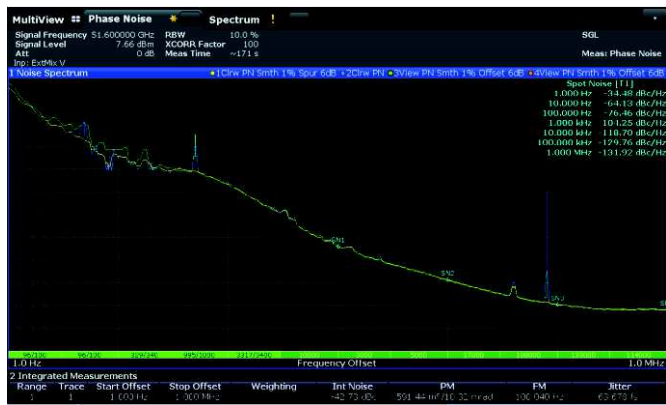
Figure 7: Measurement at 25.8 GHz shifted by 6 dB (green) and measurement at 51.2 GHz (yellow)
