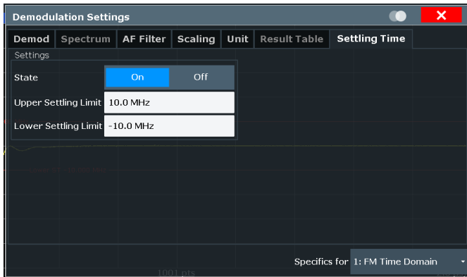
Fig. 9: Settling time tab within the demodulation configuration dialog
