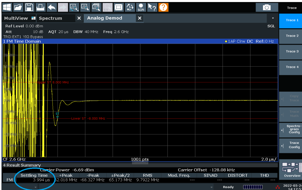
Fig. 10: Result screen of the settling time measurement
