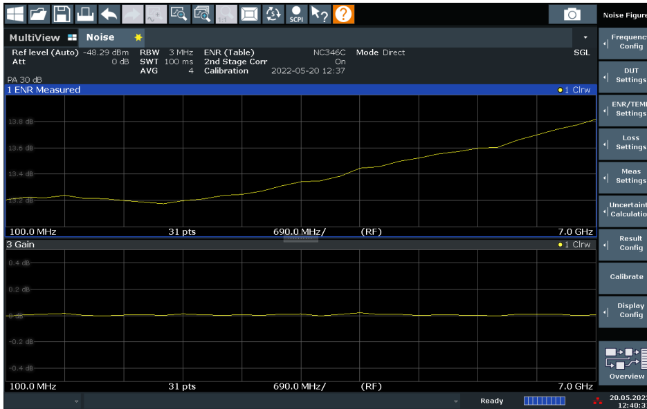
Figure 7: Measured ENR and Gain after the calibration
