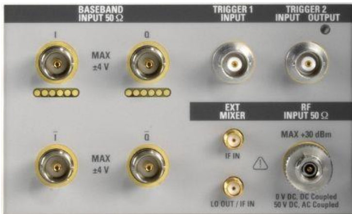
Figure 12: Baseband and Probe inputs on the R&S FSW spectrum analyzer front panel
