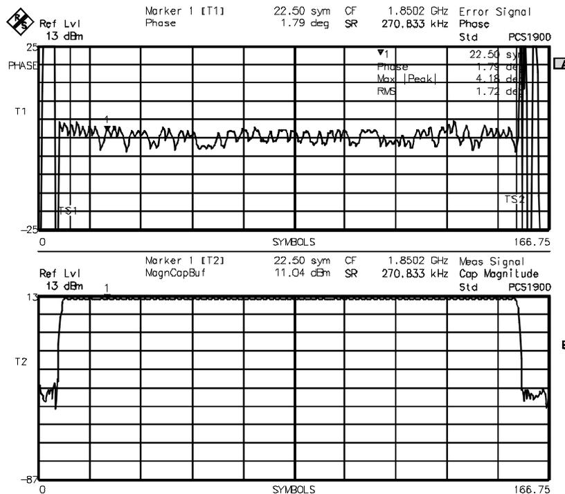
Fig 1 Display of PCS1900 phase error measurement
