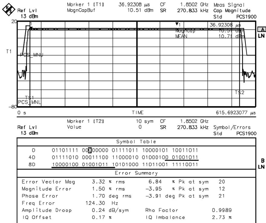
Fig 2 Display for power vs. time measurement and Mean Power in vector analyzer mode
