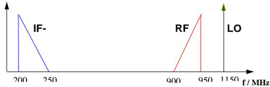
To configure the inverse sweep direction of the receiver in the ARBITRARY table, the fundamental frequency range is converted into the negative range by subtracting the frequency span of 450 MHz. The ZVR will display the fundamental frequency range (200 MHz to 250 MHz) on the x-axis.
