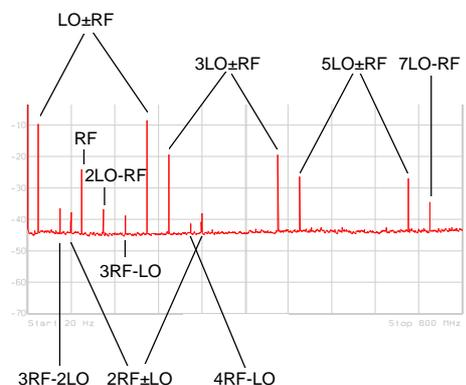
Fig. 2: Typical output frequencies on a mixer measurement.
