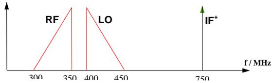
In this case, the external generator has to sweep in inverse direction. To configure this measurement, from the fundamental frequency (equal to RF), which varies from 300 MHz to 350 MHz, the LO frequency range, varying from 450 MHz to 400 MHz must be derived. A (formal) negative frequency value causes the ZVR source to sweep in inverse direction. In this case, the negative sign is generated by subtracting 750 MHz from the fundamental frequency.
