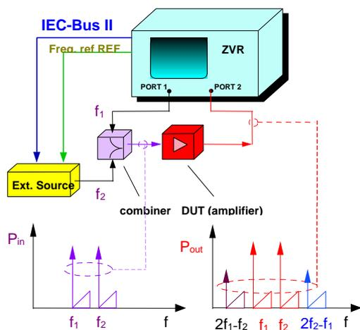
Fig. 4: Test setup for an amplifier measurement: To measure the intermodulation, a two tone signal is produced using a combiner.
