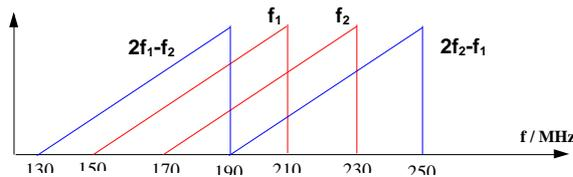
The frequency range of the lower signal  $f_1$  should be displayed on the x axis and thus be equal to the fundamental frequency F:
