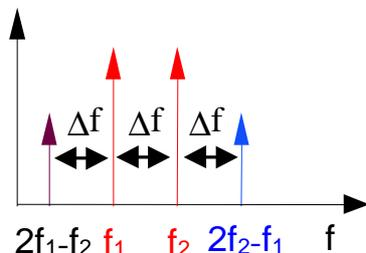
Fig. 5: Relationship between two carriers  $f_1$  and  $f_2$  and their intermodulation products  $2*f_2-f_1$  (upper IP3) and  $2*f_1-f_2$  (lower IP3). The distance between all adjacent frequencies is constant and equal to  $\Delta f=f_2-f_1$ .
