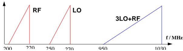
The parameters for the ARBITRARY table can be derived as described below. The frequency range of the mixing product should be displayed on the x-axis and so be equal to the fundamental frequency F:
