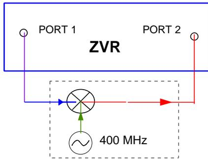
Fig. 7: Block diagram for a measurement on a mixer with internal LO generator, symbolised by the dashed line. LO frequency e. g. 400 MHz. In this example, the internal LO can be simulated using an external signal generator, which is not controlled by the ZVR but manually configured.
