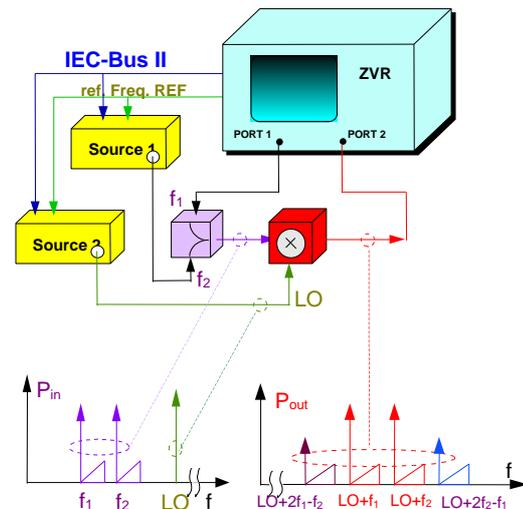
Fig. 6: Test setup for an intermodulation measurement of a mixer: To provide a two tone signal and a LO signal, a second external signal generator is used.
