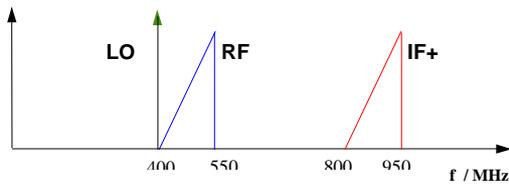
To perform this measurement, it is sufficient to sweep just the source and the receiver of the ZVR with a constant offset of 400 MHz.
