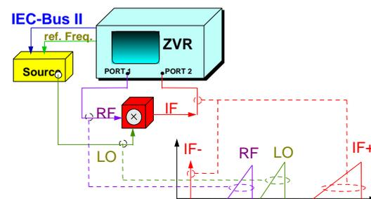
Fig. 3: Test setup for a mixer measurement, consisting of a ZVR, a second signal source (external signal generator), a mixer and IEC bus, control and RF cables.
