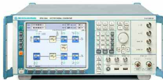
Figure 1: As top-class, the SMU200A Vector Signal Generator can combine two complete RF and baseband paths at a frequency up to 6 GHz in the first path and 3 GHz in the second path. Together with the SMU-K49 Digital Standard 802.16 option, it is the ideal instrument for generating two independent 802.16 signals to perform all necessary receiver tests - with only a single instrument.
