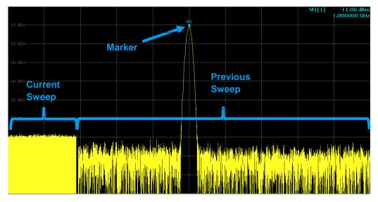
The following figure shows a spectrum measurement, where the sweep time was changed between two sweeps.
