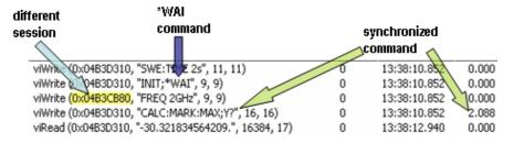
Note that \*WAI does not affect the communication with other instruments. In the example above, the frequency setting of a second instrument is performed immediately after the initiation of the sweep. The marker search operation however, is delayed for 2 seconds, because the sweep time was set to this value.
