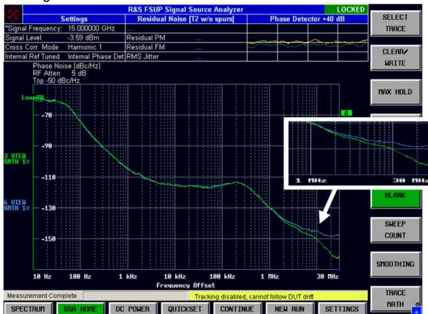
Figure 7: Phase noise measurement of signal generator R&S SMF at 15 GHz using a divider (blue) or the cross correlation extension R&S FSUP-B61 (green). The blue trace shows, that at offset frequencies > 1 MHz the sensitivity is limited by the residual phase noise of the divider.
