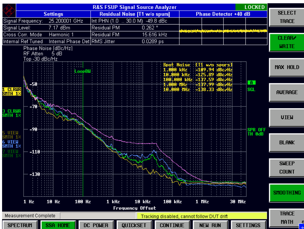
Figure 3: Measurement of a very clean microwave source without cross correlation (pink), with about 100 (blue), 1000 (green) and 20000 (yellow) averages at 25.2 GHz.
