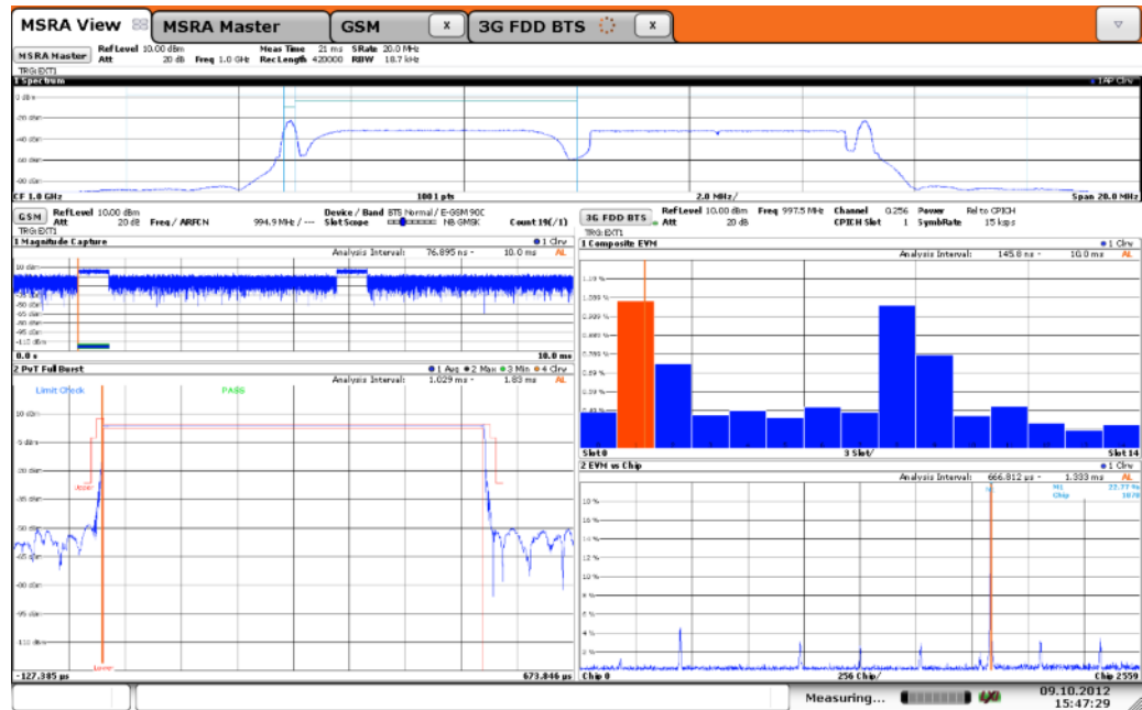
Figure 7: MSRA View of MSR signal with time correlations
