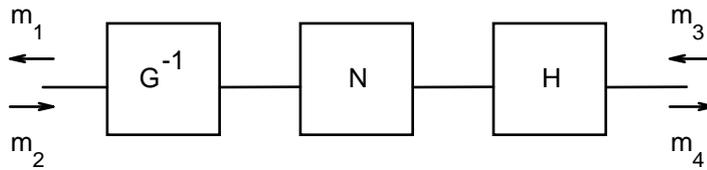
Figure 3: Cascaded network of two error two-ports and the device-under-test.
