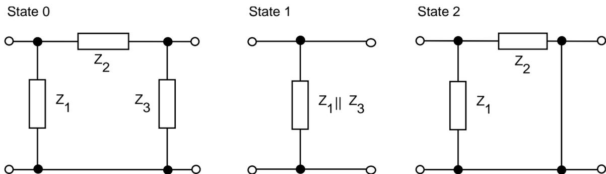
Figure 11: Switching states of the pi-network
