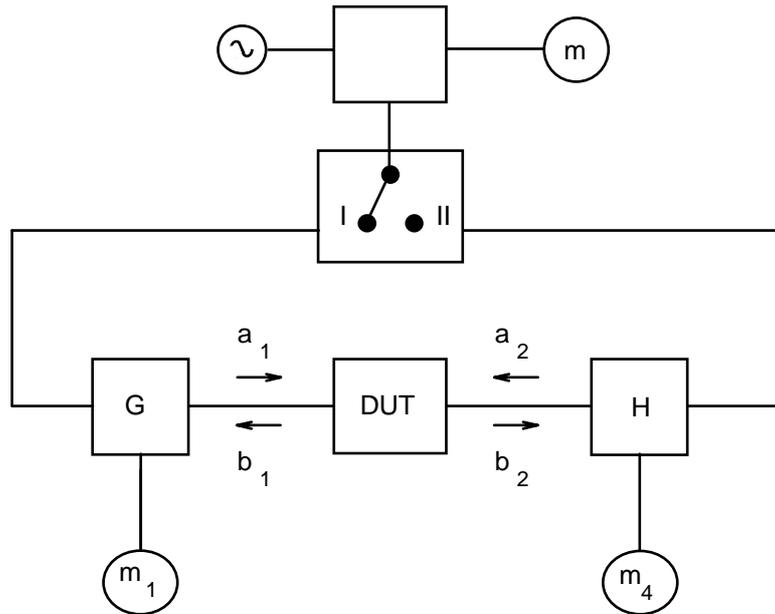
Figure 9: Block diagram of a vector network analyzer with three receiver channels, e.g. ZVRE
