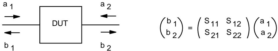
Figure 1: Scattering parameter description of a two-port device.
