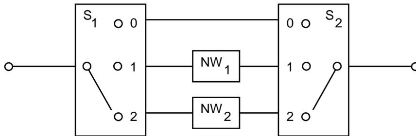
Figure 12: Realization of the switching network.
