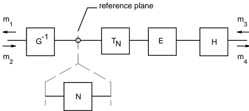
Figure 6: Realization of virtual calibration standards.
