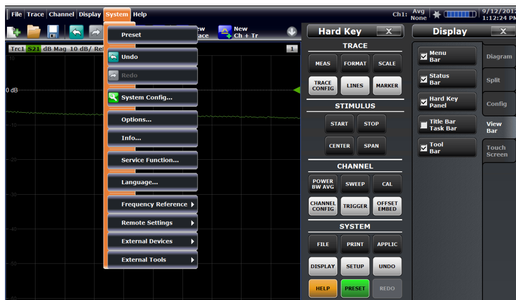
Figure 5 - Making the "Hard Key" panel visible and two methods of instrument "Preset".
