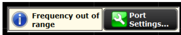
Figure 3 - Warning message after connecting NRP-Zxx power sensor Selecting “Port Settings...” opens a window, as shown in Figure 4.
