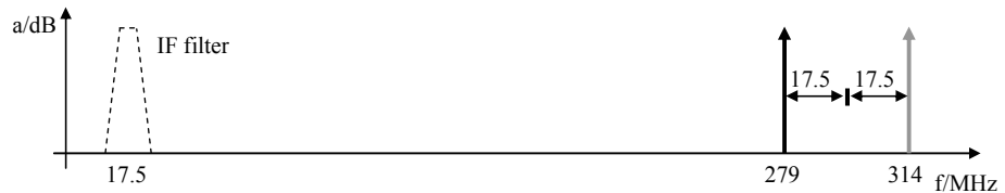
Fig. 4.28: Wanted-frequency und image-frequency reception for f_{LO\_ZVA} < f_{RF}
