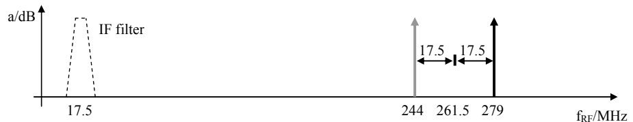
Fig. 4.29: Wanted-frequency und image-frequency reception for f_{LO\_ZVA} > f_{RF}
