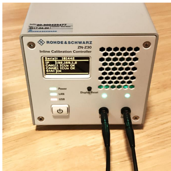
Figure Fifteen. Front panel of the ZN-Z30 controller showing the IP address.
