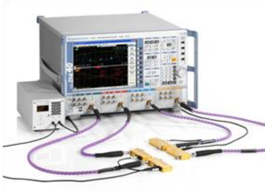
Figure Five: A complete solution consists of a VNA with a corresponding ICU connected to each VNA port. The Controller is connected to the VNA with a LAN cable, and to each ICU with a CAN bus cable. The system is controlled by the Inline Calibration Tool (Software), whose User Interface is shown at the top.
