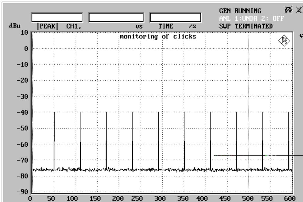
Fig. 2: Clicking noise simulated with the aid of  $\text{sin}^2$  pulses
