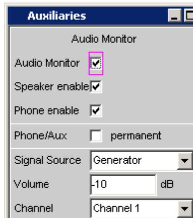
**Figure 6: Monitor settings in the Auxiliaries panel**
