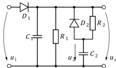
Fig. 2-10: Schematic simulating the nonlinear decay of the core loudness (ISO, 2017-06)
