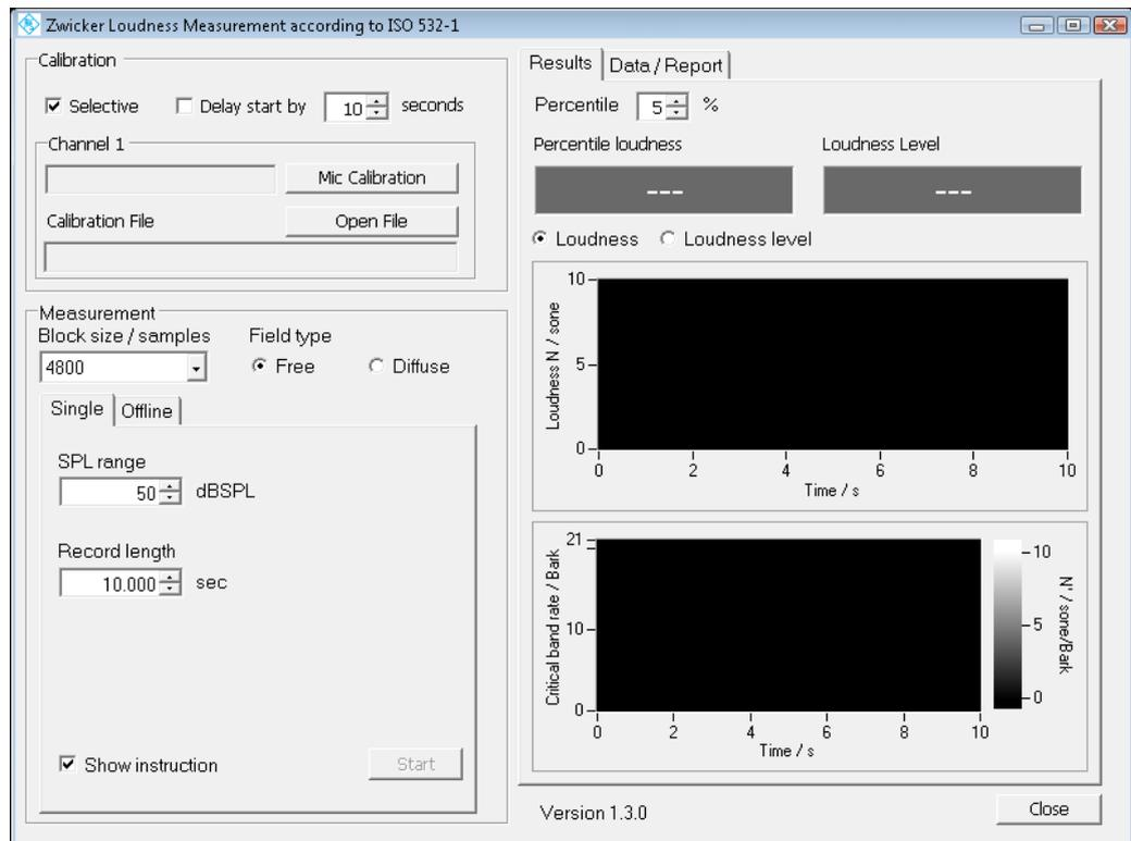
Fig. 4-1: Main window of the application program
