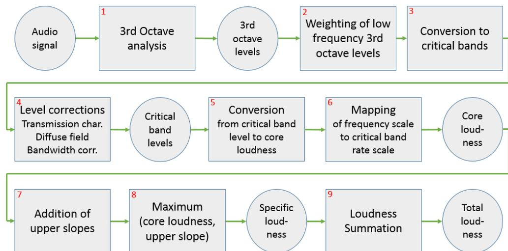
**Fig. 2-6: Block schematic of the loudness calculation process for stationary sound**
