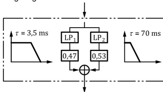
Fig. 2-11: Structure for the temporal weighting of the total loudness (ISO, 2017-06)
