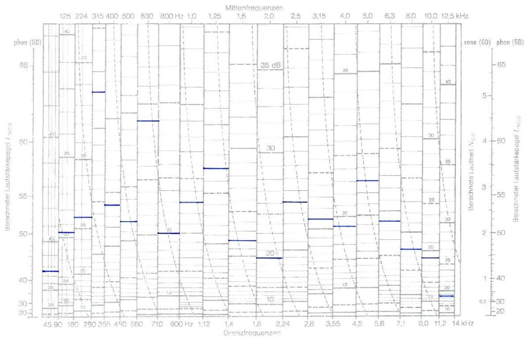
Fig. 2-7: Loudness calculation template from (DIN, 1991-03) with core loudness (blue)
