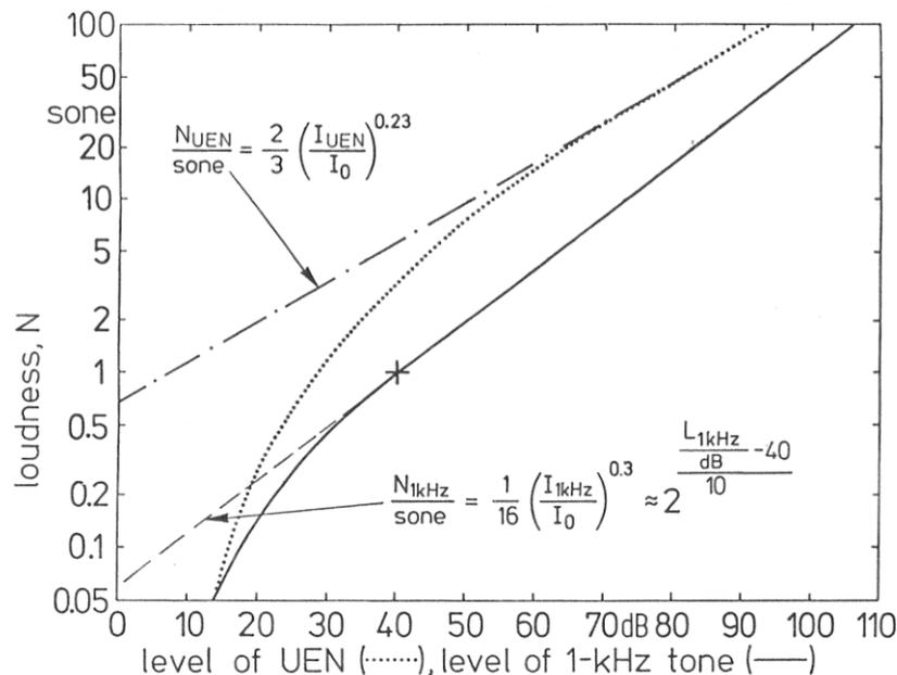
Fig. 2-5: Loudness function of a 1 kHz-tone (solid line) and of broadband “uniform-exciting” noise (dotted). From (E. Zwicker, 1990).
