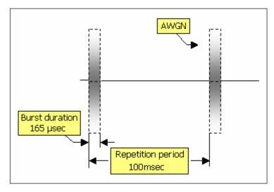
Figure 6: Impulsive noise burst as specified in document A/74:2010
