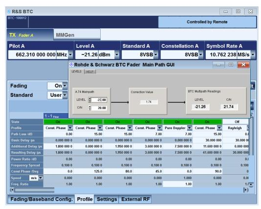
Figure 8: Fading settings for single static echo test including main path level correction.
