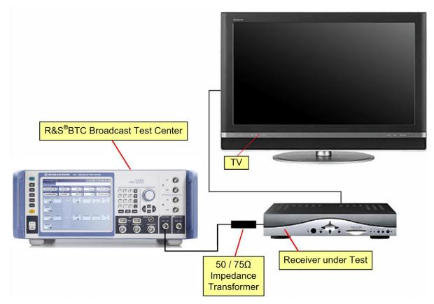
Figure 1: Receiver sensitivity test setup
