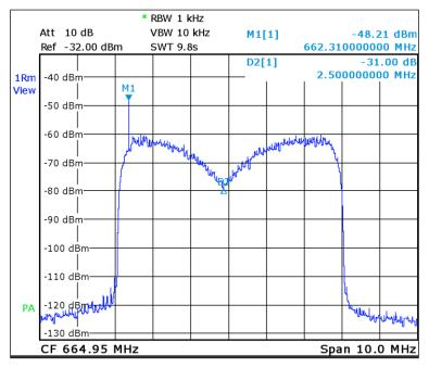
Figure 9: Resulting notch position for an echo delay of 0.2  $\mu$ s.
