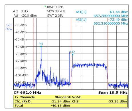
Figure 5: Wanted ATSC signal with lower adjacent NTSC signal
