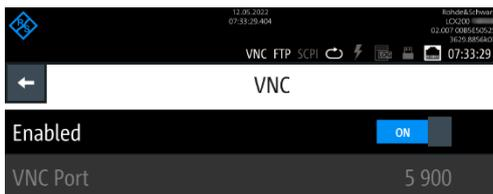
Figure 4-1 VNC configuration subitem in the device menu
