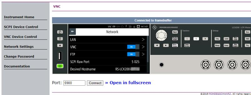
Figure 3-3 VNC device control page of R&S®LCX200
