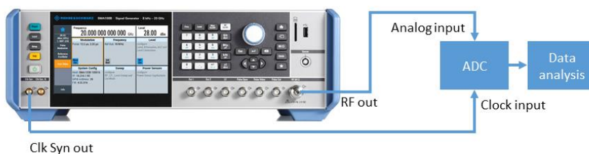
Figure 33 Simplified ADC test setup using the R&S®SMA-B29 clock synthesizer as clock source
