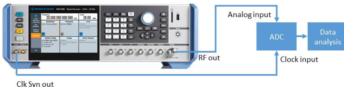
Figure 2 Modern ADC performance test setup
