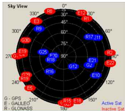
Fig. 13: Sky view display of the SMBV showing the satellites visible in the sky.
