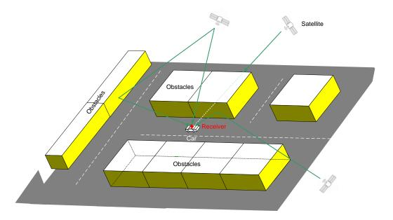
The SMBV automatically simulates the multipath propagation caused by the defined obstacles based on the satellite constellation, receiver position (and movement), and even surface material of the obstacles. A detailed description of this feature can be found in reference [7]. Please see this dedicated application note for further details.
