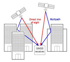
For testing the receiver's multipath mitigation performance, the SMBV can simulate multipath propagation in two ways:
