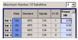
In this example, each satellite signal will have a level of –130 dBm, and four satellites together will have a level of four times –130 dBm, which equals –124 dBm [4].
