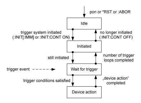
Other emulated instruments and also the SMF implement the trigger control system shown in the following figure:
