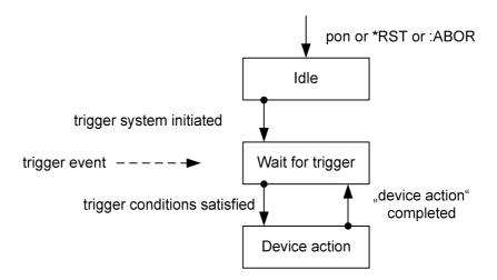
The main difference between the emulated instrument's and the SMF's trigger control system is that there is no "Initiated" state in the SMF. The SMF implementation assumes that the trigger system is initiated automatically in the "Idle" state. As a result, any sweep operation in the SMF, once activated, can only be controlled by internal or external trigger events.
