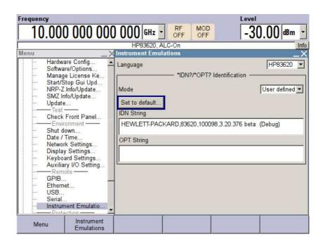
Then select the IDN String text box and edit the response text to \*IDN? queries. When finished, confirm the text:
