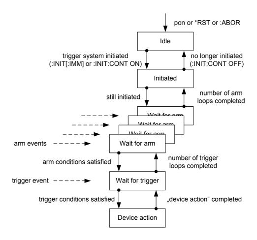
Some of the emulated instruments implement a simplified trigger control system:
