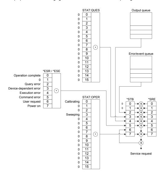
Some of the emulated instruments implement a more detailed status and error reporting system. Since the additional information stored in that system is not available in the SMF, application code that uses the additional information must be changed.
