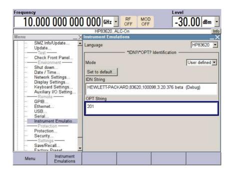
Finally select the OPT String text box and edit the response text to \*OPT? queries. When finished, confirm the text:
