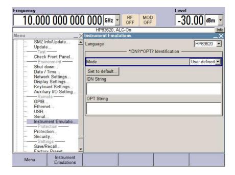
In "User defined" mode, press the "Set to default..." button to preset the corresponding IDN string and/or OPT string text boxes with the default settings from the selected remote emulation:
