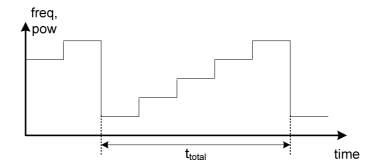
Changing the start, stop or steps parameter of the sweep operation does not have an impact on the total sweep time.
