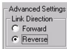
Link Direction activates the downlink channel (Forward - from base station to mobile station) or the uplink channel (Reverse - from mobile station to base station). The setting influences both channel frequencies and slot type.
