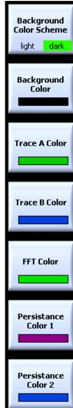
The first button changes the background color scheme between a dark setup and a light setup. A dark setup may be ideal for viewing the data on a computer screen, while a light setup is a better choice for printing the results or for placing a screenshot in a document.
