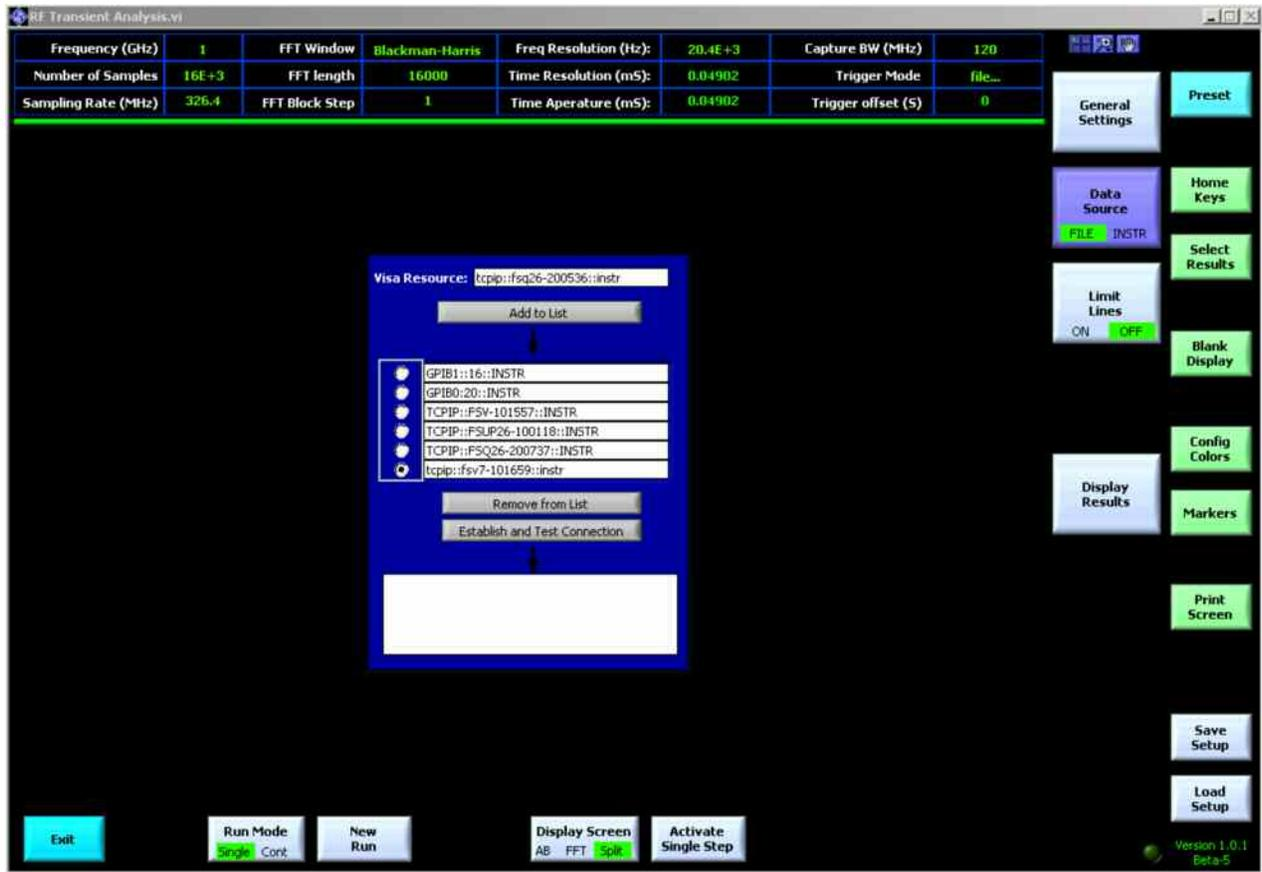
Successive presses of the Configure Interface softkey will toggle the option of acquiring the IQ data from a spectrum analyzer, or using previously captured IQ data that has been stored in a file.
