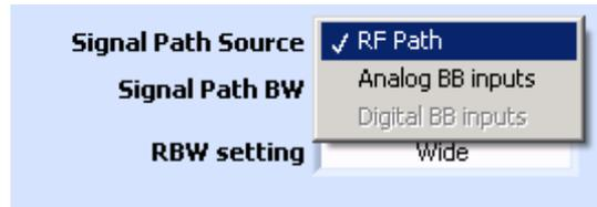
This variable controls the input of the spectrum analyzer. The choices are the RF input, the base band analog IQ inputs, and the base band digital IQ inputs. The digital IQ input option is not functional in this initial release of the RF Transient Analysis software.
