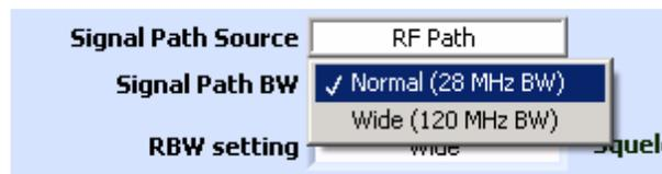
This variable controls the IF path of spectrum analyzers that have multiple ADCs. For example, the FSQ has a 28 MHz wide IF path the first set of ADCs, and also a 120 MHz wide IF path for a second set of ADCs.
