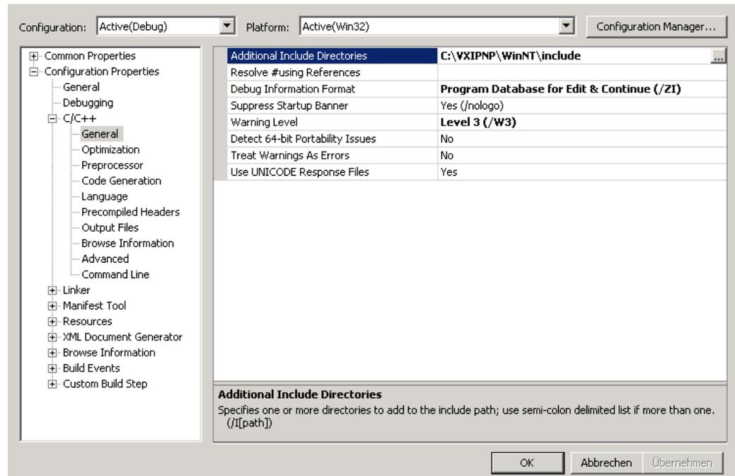
Figure 8: C++ Compiler settings for instrument driver header files.
