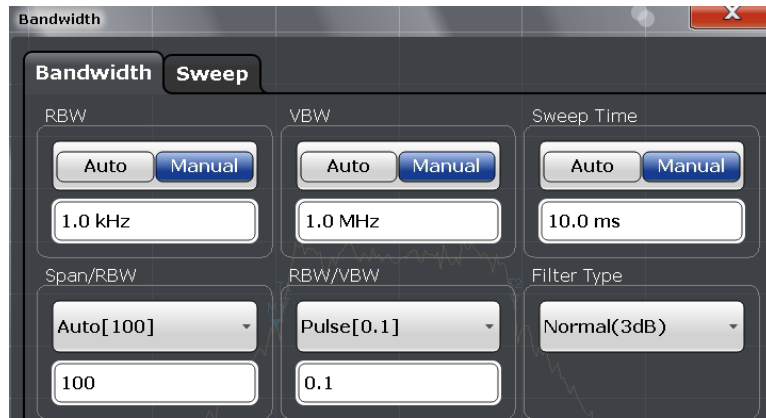
Fig. 3-95: OBW: set the bandwidth and sweep.
