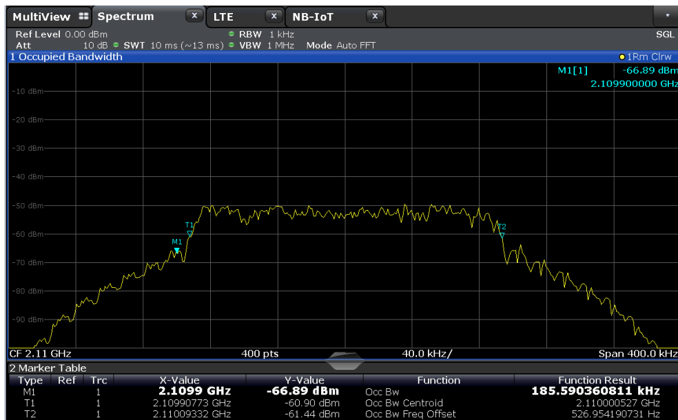
Fig. 3-96: NB-IoT OBW measurements.
