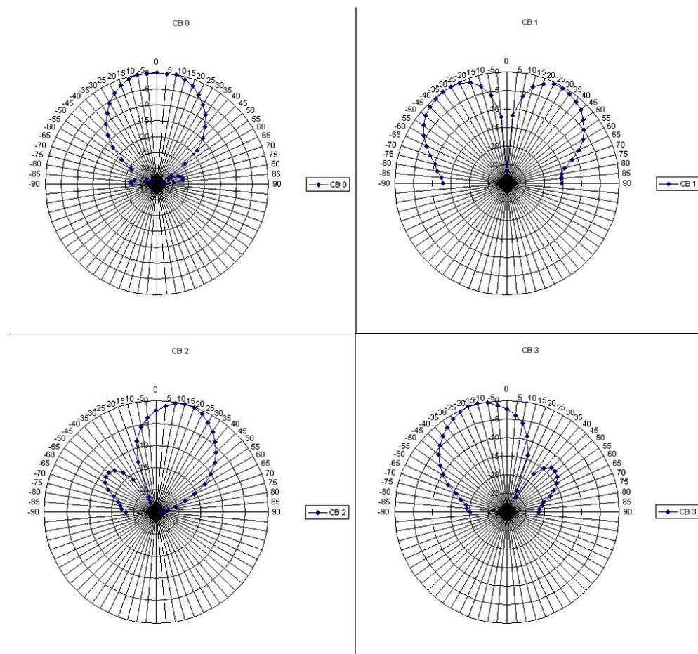
**Fig. 3:** Schematic representation of TM 6t for two antennas at a distance of  $\lambda/2$ , codebook index 0 to 3.
