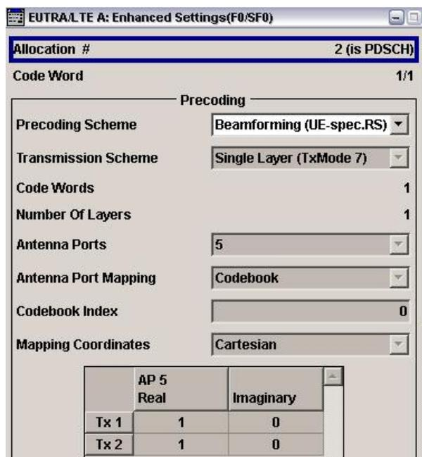
Fig. 45: Display of the beamforming settings in the allocation; this example shows TM 7 on AP 5 with codebook 0.
