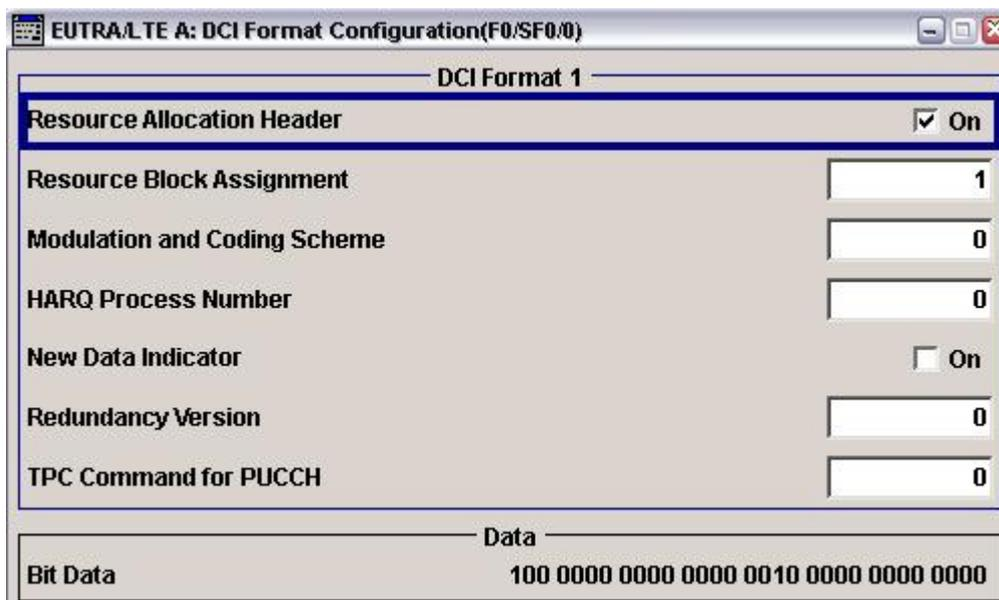
Fig. 38: Example configuration of DCI format 1 for TM 7.
