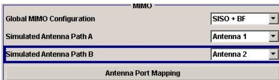
*Fig. 59: Settings for SISO beamforming. Cell-specific reference signals are generated for one antenna in this case. Only the PDSCH receives differing phases.*
