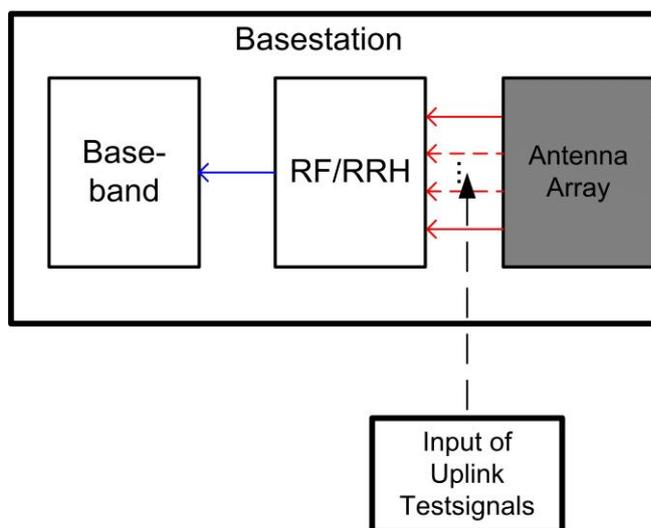
Fig. 25: Block diagram for base station receiver tests: Generation of the uplink signals on the RF module.
