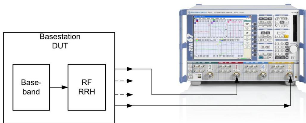
**Fig. 22: Transmitter test setup with the ZVx network analyzer. Depending on the model, up to eight RF paths can be measured simultaneously.**
