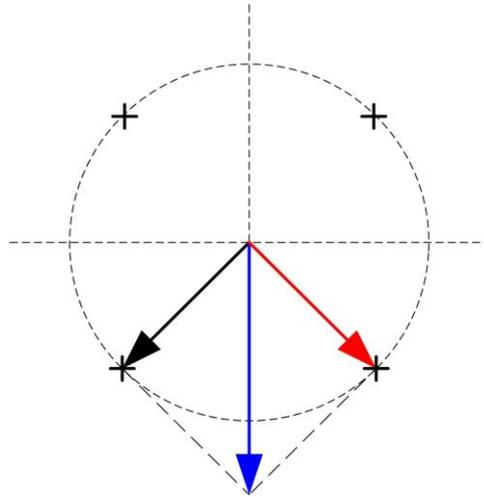
**Fig. 6: Example of the weighting of two signals (here with a phase difference of 90°).**
