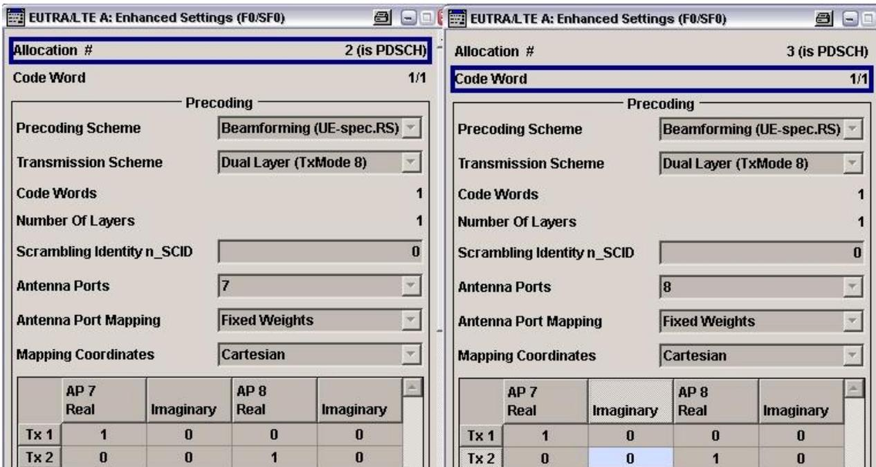
Fig. 57: Different antenna port (AP) settings in Dual Layer Beamforming for Multi User
