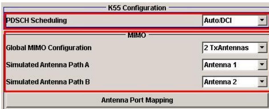
Fig. 34: Number of antennas and assignment to the individual basebands in the SMU.
