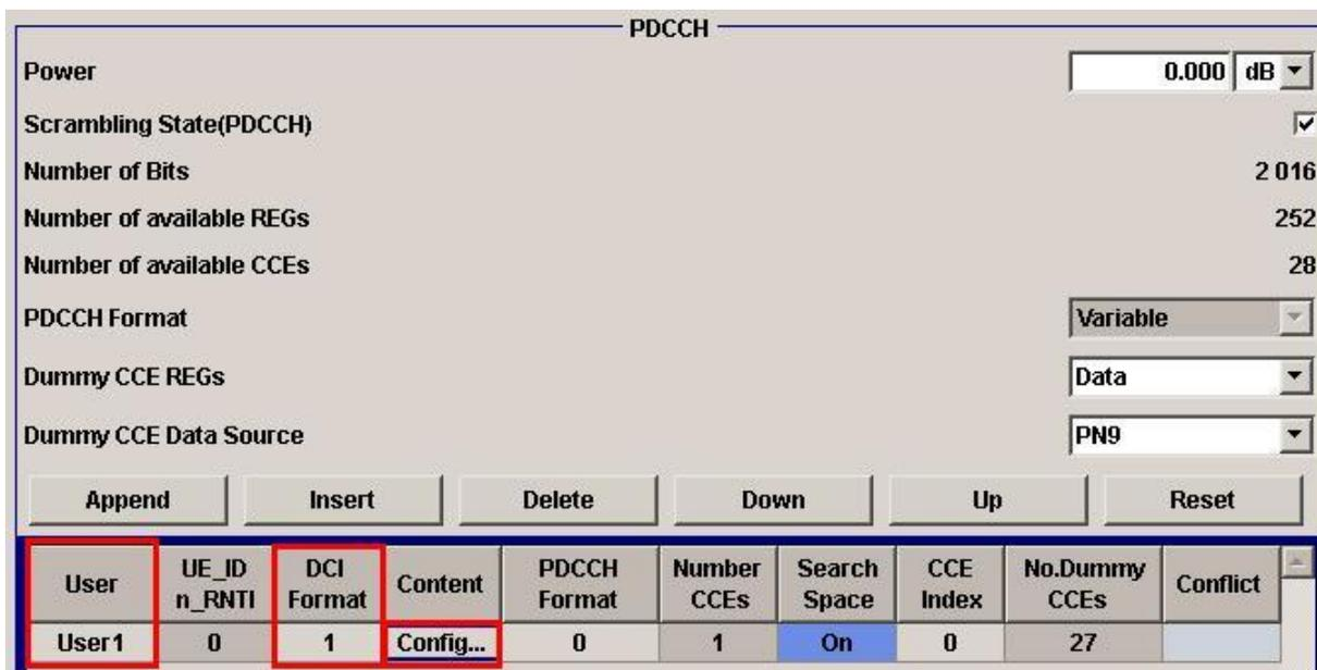
Fig. 37: Setting the DCI format in the PDCCH for TM 7: DCI format 1.
