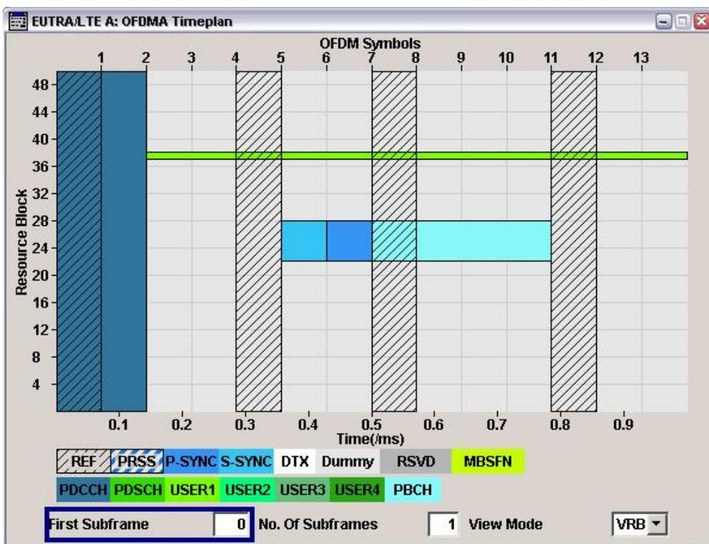
Fig. 40: Display of the OFDMA timeplan parameters that are set automatically in AUTO/DCI mode.
