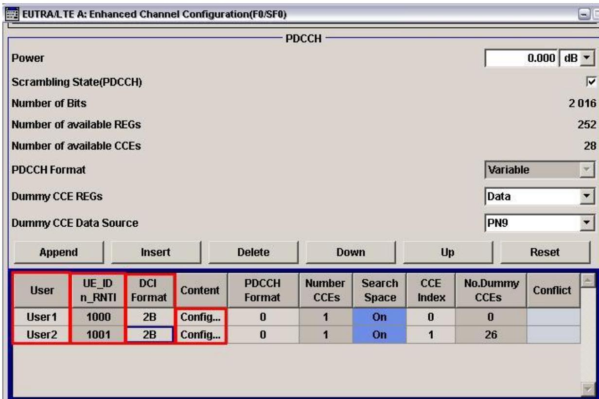
Fig. 55: Setting the DCI format in the PDCCH for TM 8 with two UEs: DCI format 2B.
