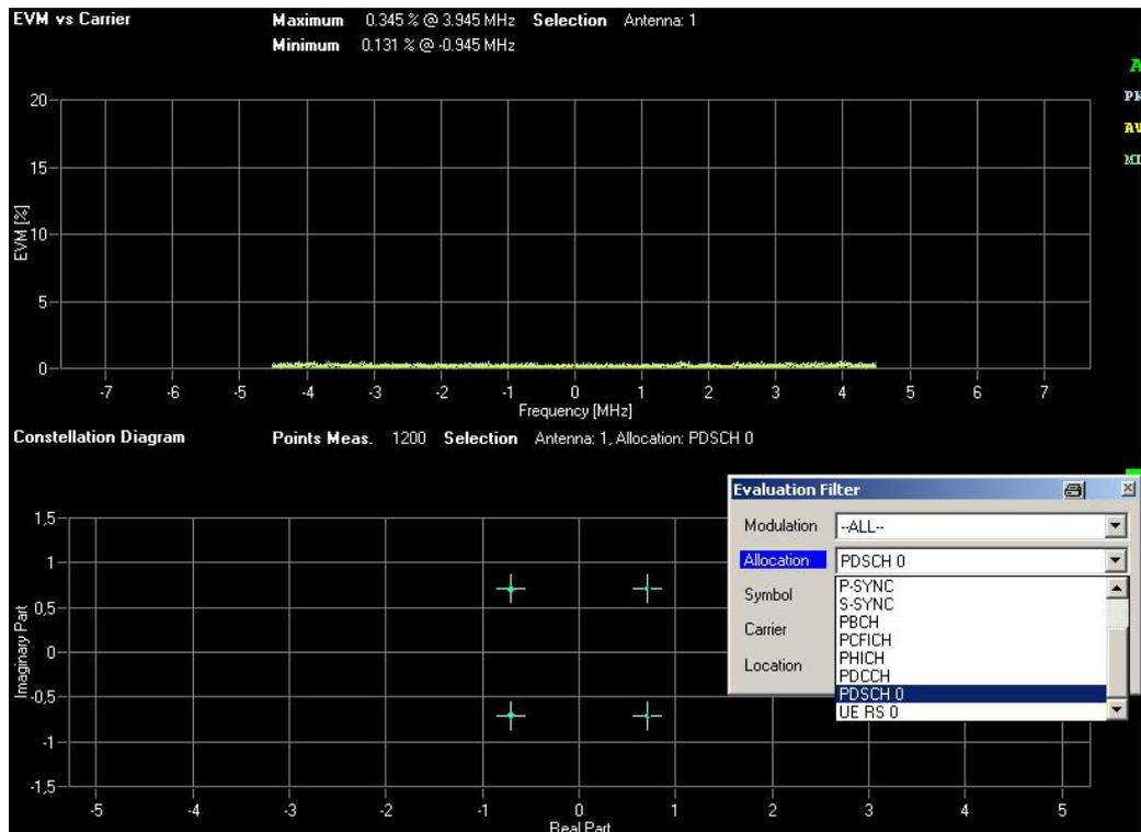
Fig. 11: EVM measurement on antenna 1 and constellation diagram of a beamformed QPSK-modulated data allocation (PDSCH) in summary.
