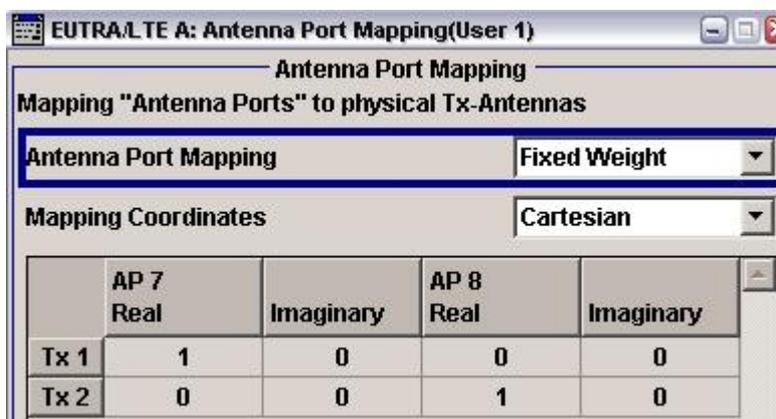
Fig. 52: Fixed weight for TM 8 with two antennas.
