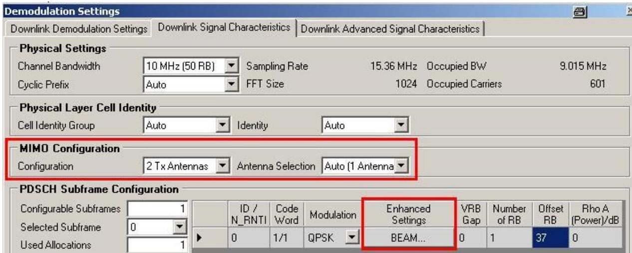
**Fig. 9: Beamforming settings in the LTE analysis software for the FSx; TM 7 in this example.**
