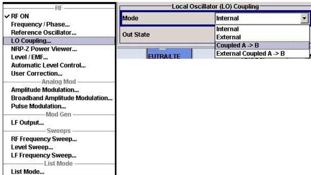
Fig. 31: Enabling phase coherence in the second RF block.
