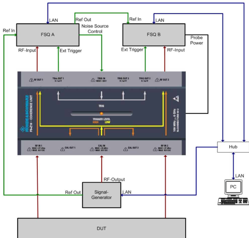
Fig. 17: Test setup for phase determination between two signals using the FS-Z10.
