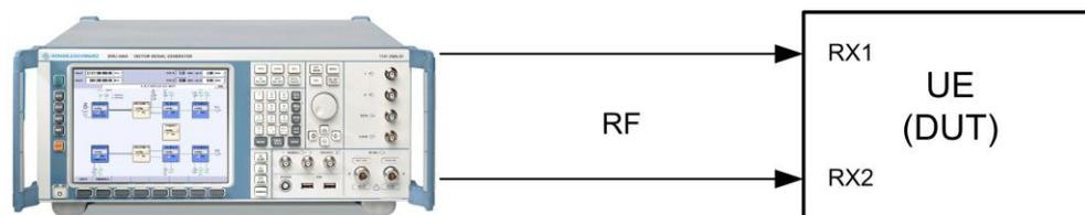
**Fig. 33: Block diagram for the UE receiver test; this example shows two antennas.**
