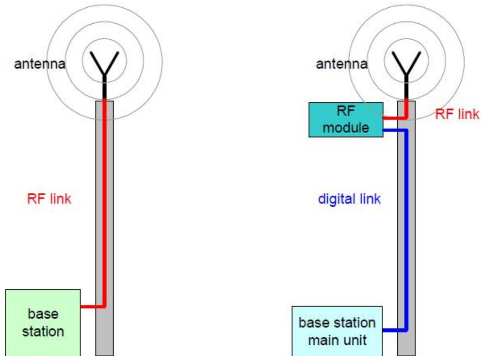
Fig. 2: Base station setup. In state-of-the-art setups, the baseband is separate from the RF module. A digital link between the baseband and the RF module is used (blue). The baseband can be located at the bottom of the mast, co-located directly on the antenna with the RF module, or placed in a completely separate location in the network.
