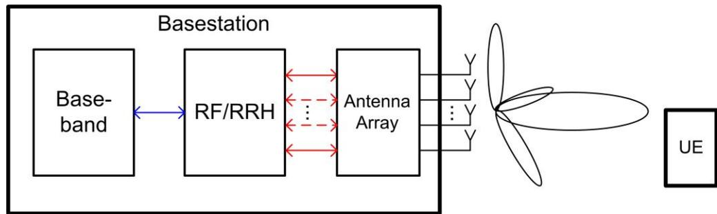
Fig. 1: Block diagram: Mobile radio transmission from base station to UE.
