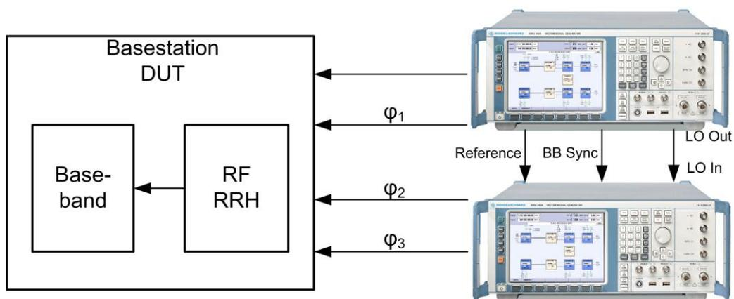
Fig. 26: Example of base station receiver test setup for four RF paths with a phase offset  $\phi$  generated by two SMUs.
