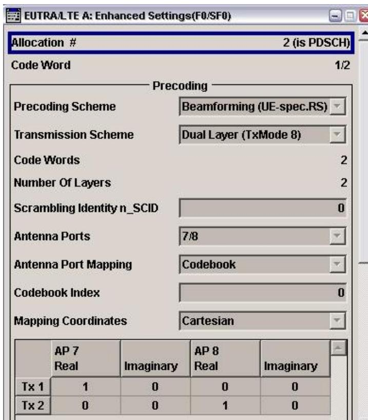
Fig. 53: Display of the beamforming settings in the allocation; this example shows TM 8 on APs 7/8 with codebook 0.
