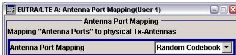
Fig. 43: Random codebooks for tests in accordance with TS36.521, section 8.3.
