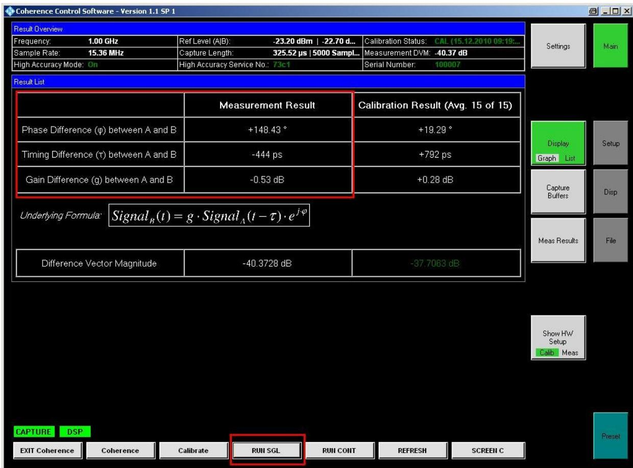
Fig. 21: Measurement using the FS-Z10: Click RUN SGL to start the measurement. The phase, timing and gain differences are displayed.
