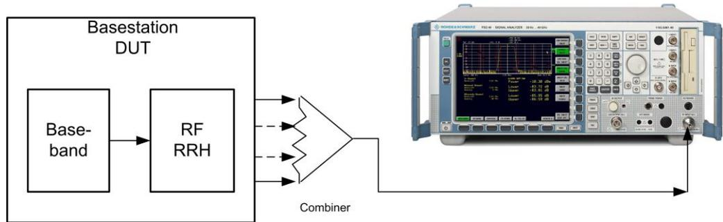
**Fig. 12: Test setup for measuring the beamforming level. All antennas are brought together using a combiner.**
