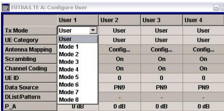
Fig. 36: Set the transmission mode in the Configure User screen. TM 7 and TM 8 apply to beamforming.
