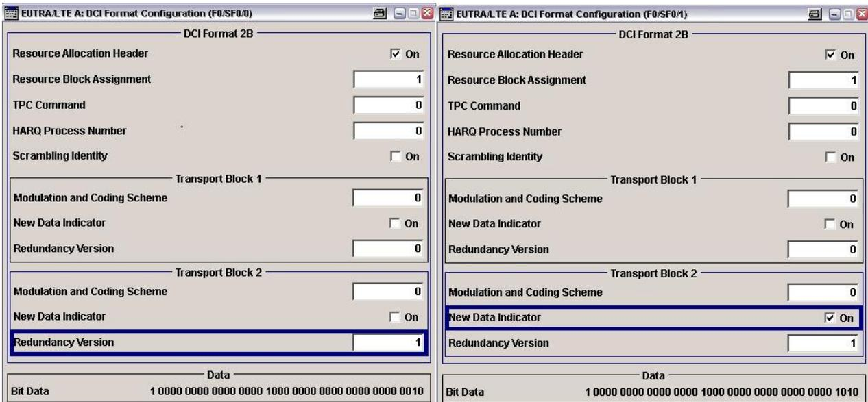
Fig. 56: Example configuration of DCI format 2B for TM 8 in multi-user mode. The second codeword (CW) is disabled by setting Redundancy Version 1. Enabling the New Data Indicator in allocation 3 sets AP8.
