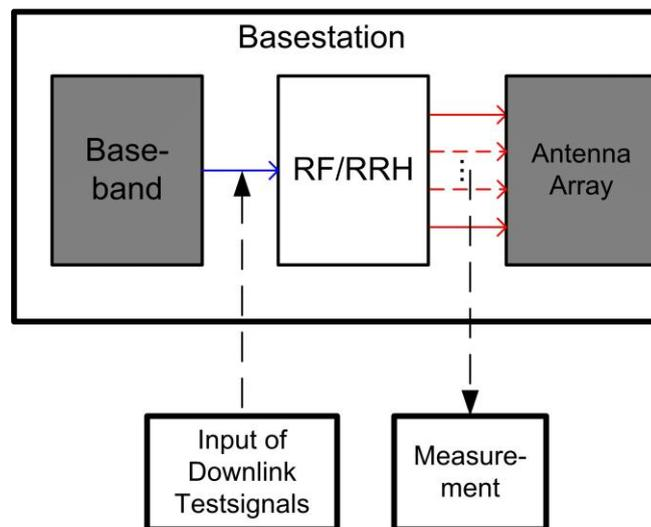
Fig. 60: Block diagram for RRH tests in the downlink.
