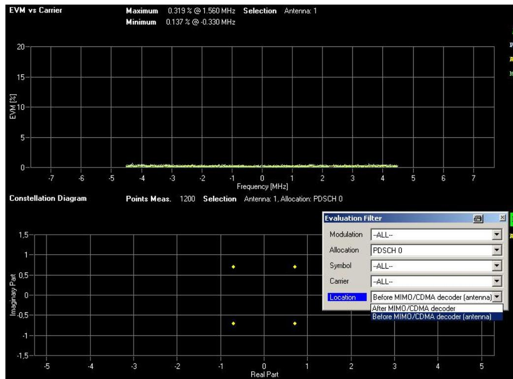
Fig. 16: Summary EVM measurement on antenna 1 and constellation diagram of a beamformed QPSK-modulated data allocation (PDSCH) in TM 8.
