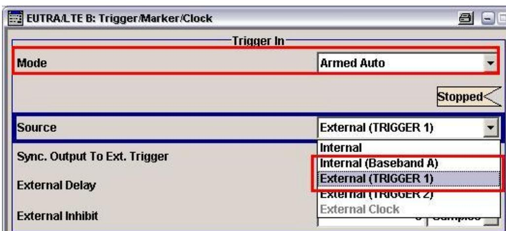
Fig. 28: Synchronizing baseband B to baseband A. Armed Auto is selected as the trigger mode, and the SMU-internal baseband A is used as the source. Enable BB A to start both BBs synchronously.
