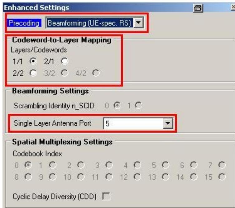
Fig. 10: Additional settings. The precoding is set to beamforming (UE-specific RS). In TM 7, a codeword is mapped to a layer at antenna port 5.
