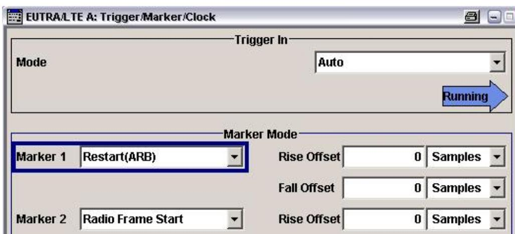
Fig. 27: BB1 marker for synchronizing the remaining basebands.
