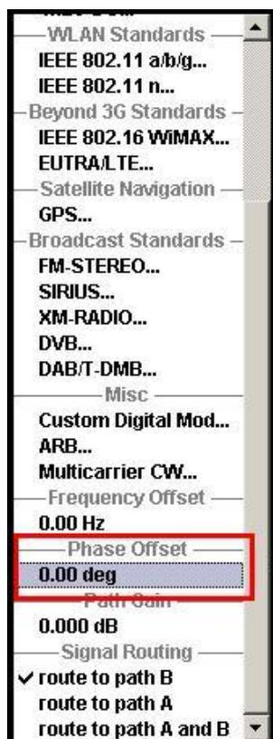
*Fig. 32: Setting a phase offset in baseband B. Both RF paths are coupled via the SMx-B90. Therefore, the phase difference results from the baseband also defined in the RF.*
