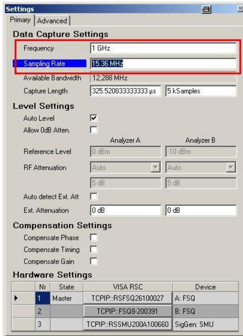
**Fig. 20: Setting the frequency and sampling rate. The sampling rate should correspond to the LTE sampling frequencies (see Table 3).**
