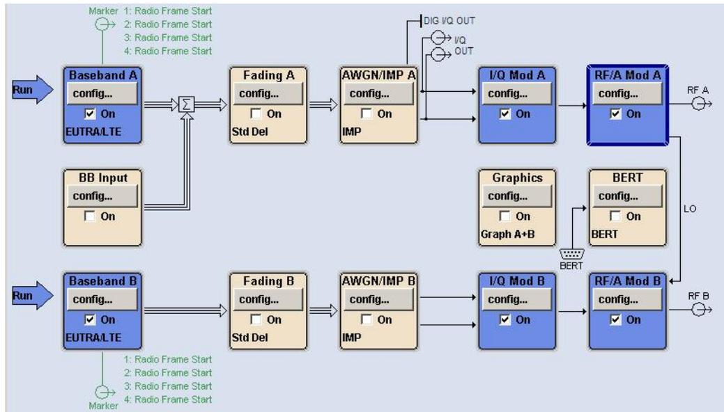
Fig. 30: SMU overview with active SMx-B90 phase coherence option. The LO line between the two RF blocks represents the coupling.
