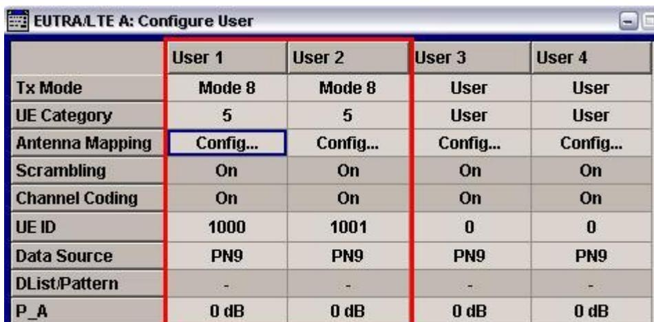
Fig. 54: Setting the users in dual-layer mode for two UEs. Note the different UE IDs.
