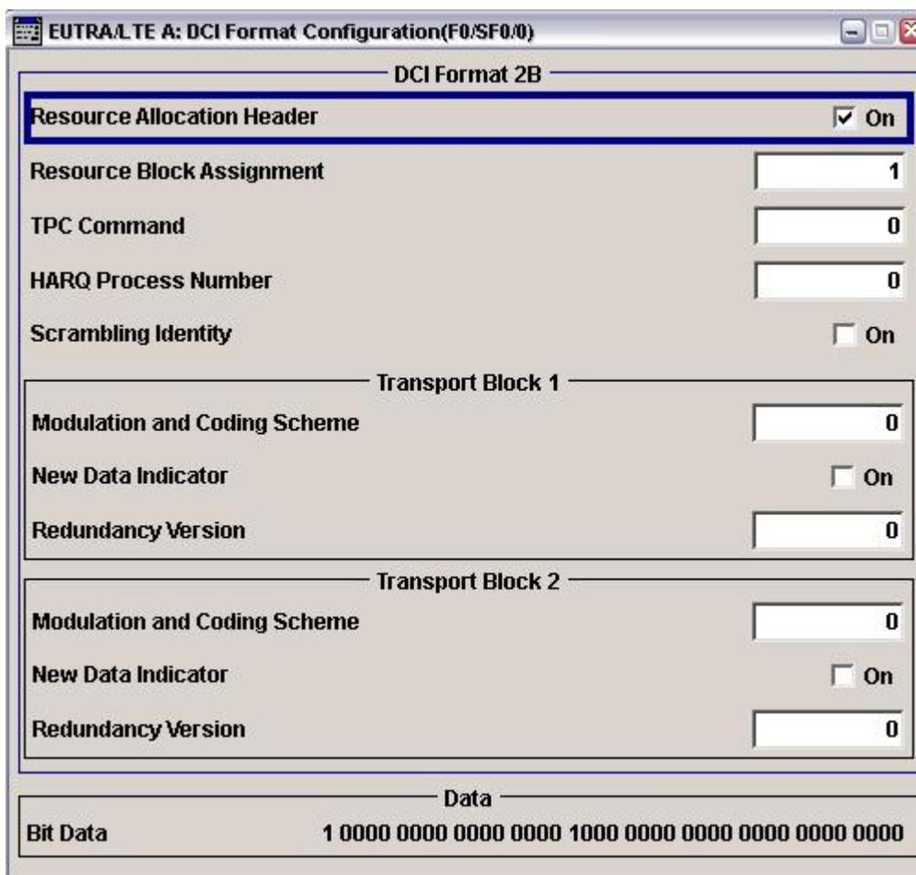
Fig. 48: Example configuration of DCI format 2B for TM 8.
