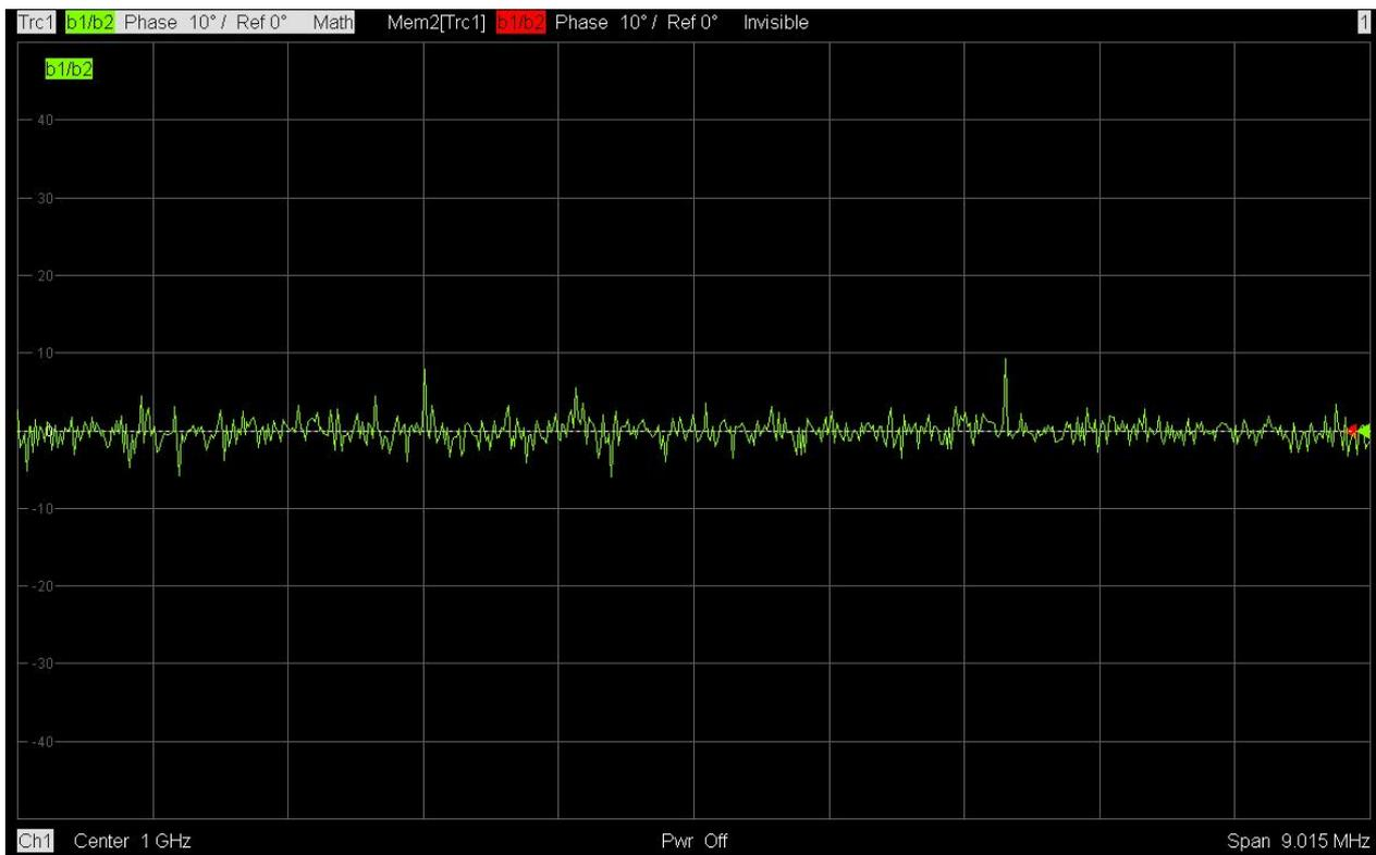
**Fig. 23: Calibrated phase trace in ZVx. The display shows the phase ratio for two LTE signals over the complete occupied bandwidth of a 10 MHz signal (50 RBs). In the example, the phase difference between the two signals is 0°.**
