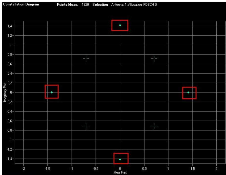
**Fig. 7: Resulting 45° phase rotation of a PDSCH allocation at a weighting of 90°.**
