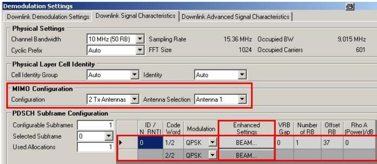
Fig. 15: Beamforming settings in the LTE analysis software for the FSx; TM 8 in this example. In dual-layer beamforming, two layers (codewords) are used.
