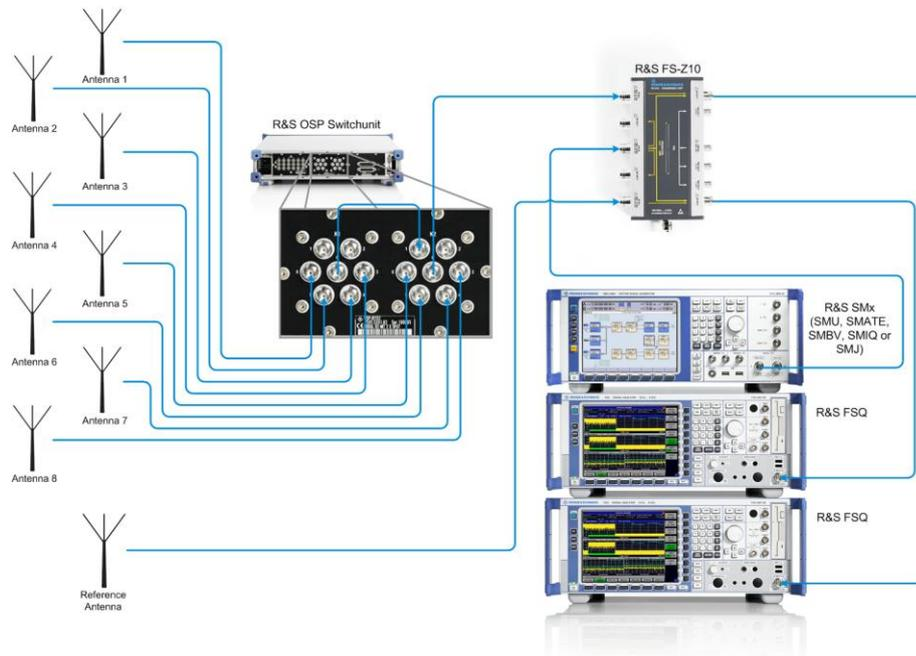
Fig. 24: Example of a test setup with the OSP.
