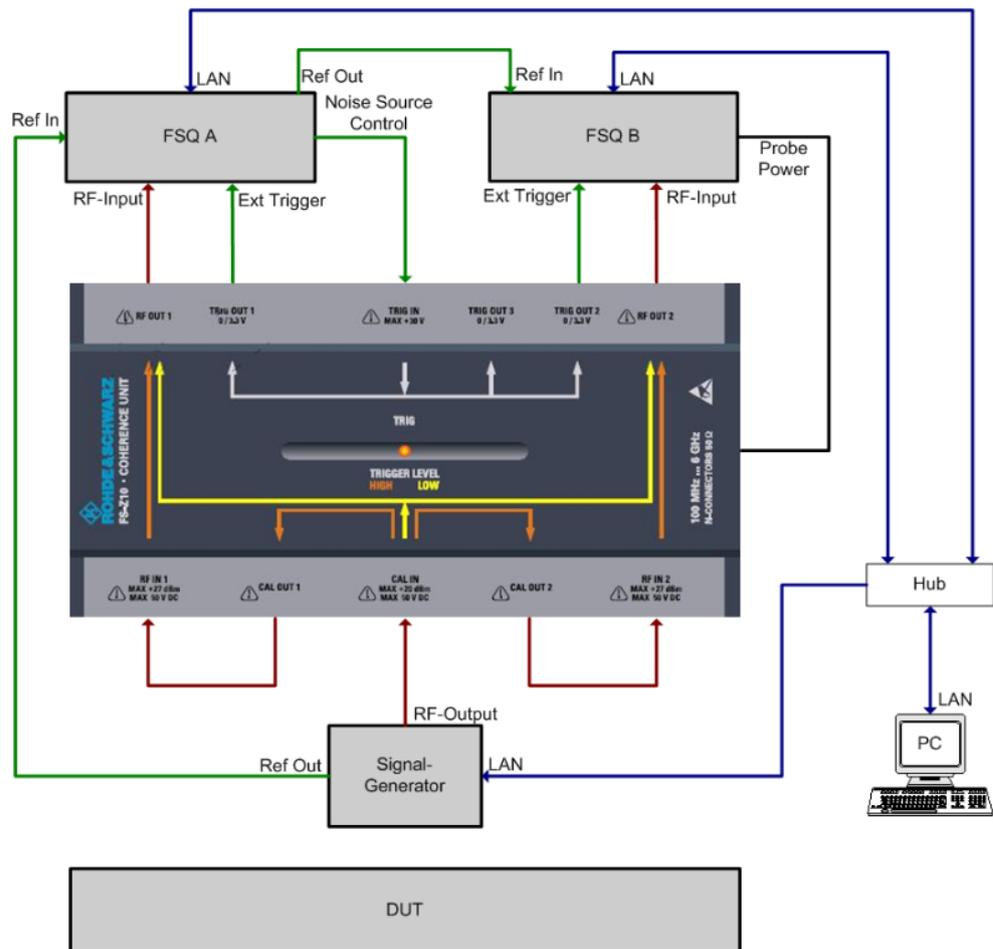
**Fig. 18: Test setup for cable calibration with the FS-Z10.**
