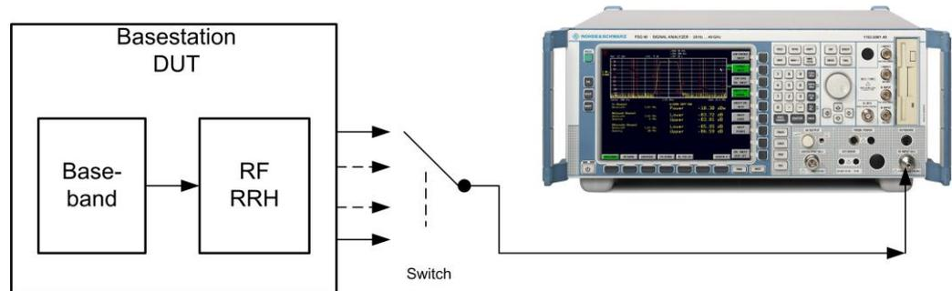
**Fig. 8: Test setup for the base station transmitter test with LTE analysis software.**
