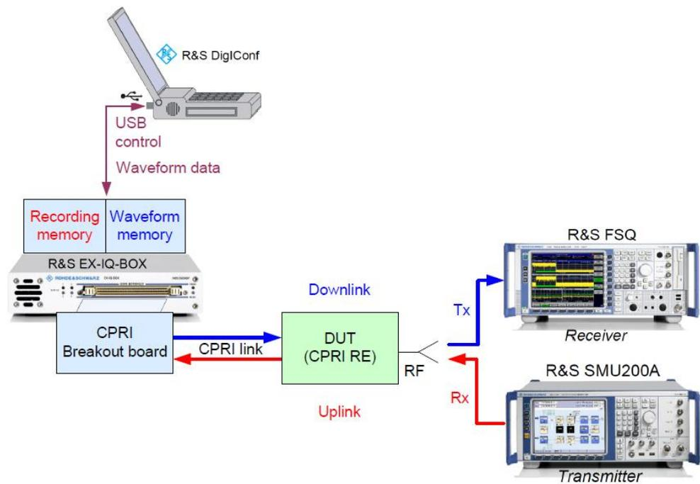
Fig. 62: RRH test setup: Bidirectional CPRI operation with standalone EX-IQ-Box.
