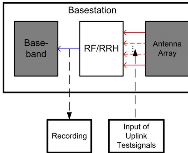
Fig. 61: Block diagram for RRH tests in the uplink.
