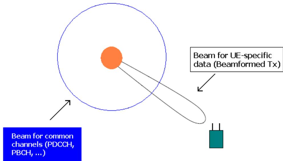
**Fig. 4: Beamforming in TM 7; use of UE-specific RS; the common channels use transmit diversity.**
