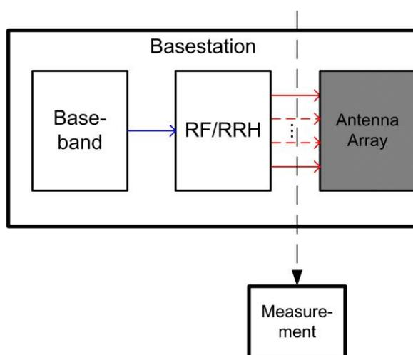
*Fig. 5: Block diagram for base station transmitter tests: Measurements are taken in the downlink on the RF module.*
