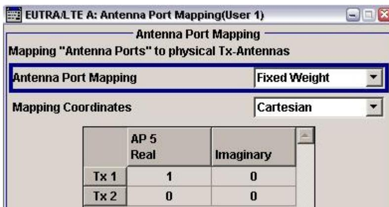
Fig. 44: Fixed weight for TM 7 with two antennas.
