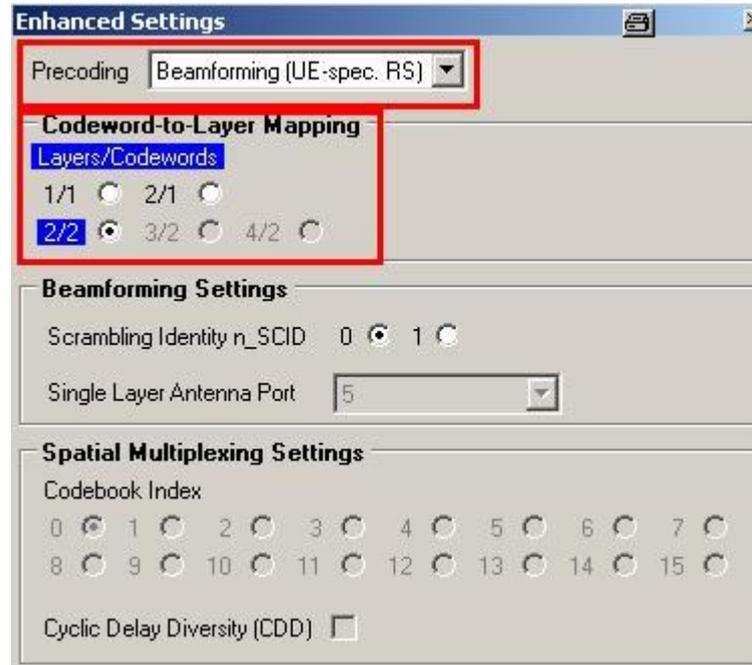
**Fig. 14: Additional settings. The precoding is set to beamforming (UE-specific RS). In TM 8, two codewords are used in two layers and mapped to antenna ports 7 and 8.**
