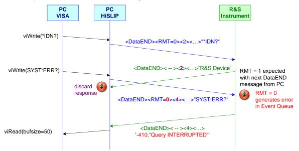
Fig. 4: Message sequence with interrupted error
