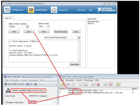
Fig. 5: Example scenario to send single SCPI commands to an instrument via HiSLIP using a VISA alias name
