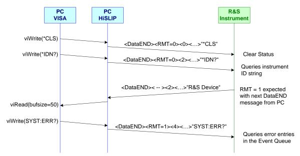
Fig. 3: Simple message sequence between controller (PC) and instrument (server)
