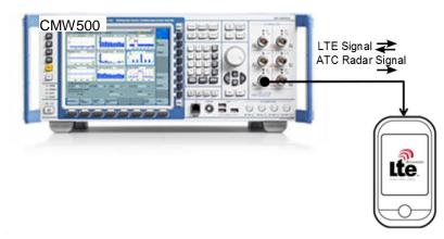
Figure 4-4: CMW500 with advanced RF frontend and DUT
