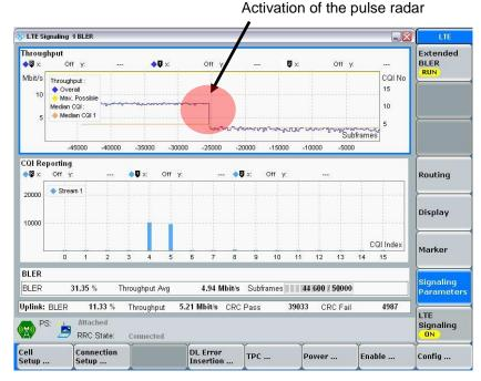
Figure 4-10: Throughput measurement when the pulse radar became active
