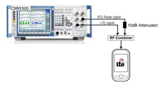
Figure 4-2: CMW500 and DUT Setup for LTE and S-Band Radar coexistence tests
