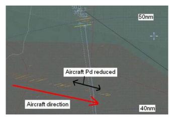
Figure 5-9: 4G Signal at 2685 MHz [9]
