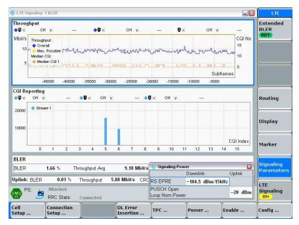
Figure 4-8: BLER Measurement and Cell Setup
