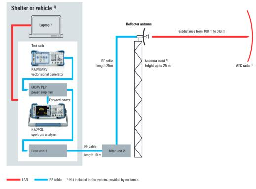
Figure 5-1: Radar Test Setup
