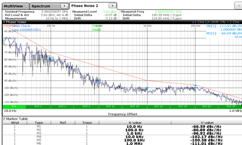
Figure 50: FSW Phase noise plot of converter under test at 70MHz IF
