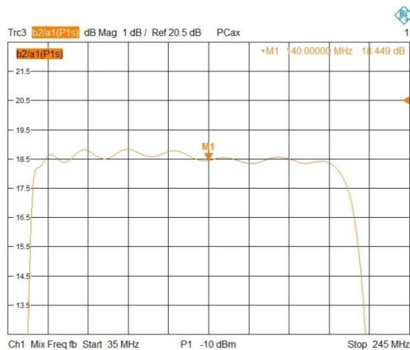
Figure 37: Conversion gain or converter under test with IF 140 MHz
