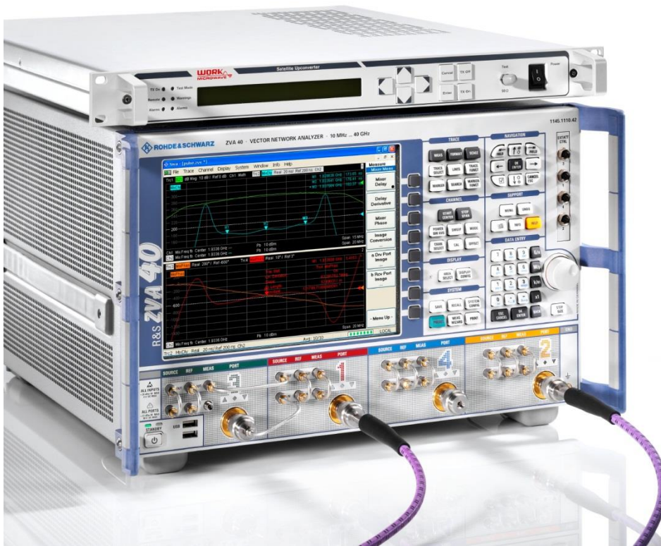
Figure 1: LO-Band satellite up-converter from Work Microwave company as device under test characterized by R&S®ZVA40 Vector Network analyzer
