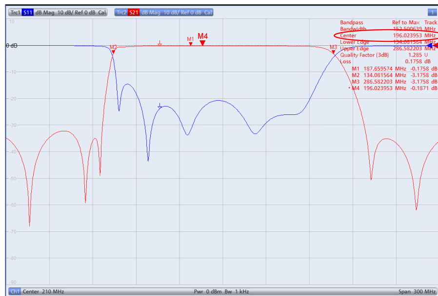
Fig. 5-9: Display of all relevant values for a bandpass.
