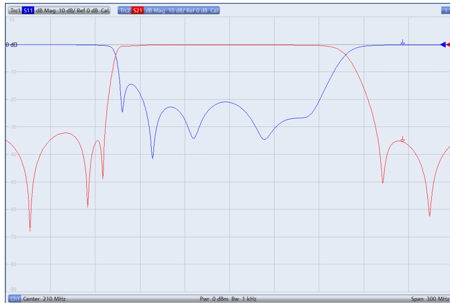
Fig. 2-31: Reflection and transmission in one diagram.
