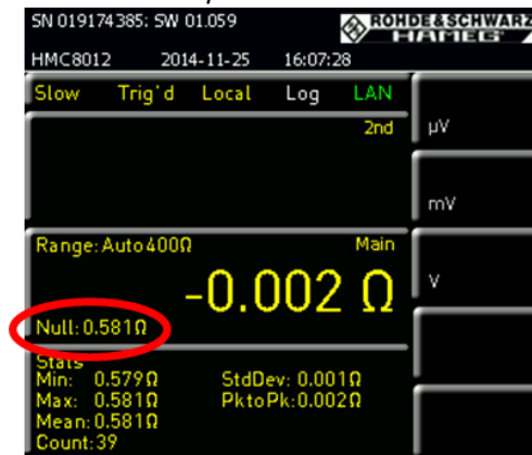
Fig. 2-11: Display of the offset value after calibration.
