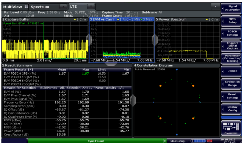
Figure 7: Measurement results on the FSW using 3-element Tx antenna with phase coherence and one receive antenna
