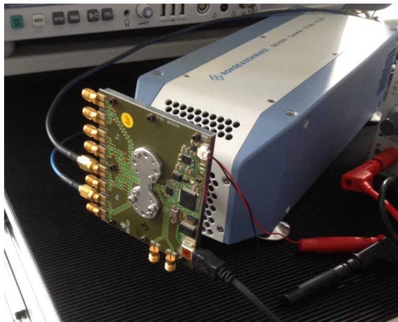
Figure 16: Photo of a practical test-setup with the SZU100A Upconverter for testing the RX part of a V-band transceiver (Supplier: "Infineon Technologies AG")
