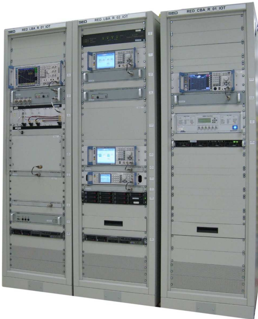
Figure 15: Automated Test System using Rohde & Schwarz Test Equipment [courtesy SED Systems]
