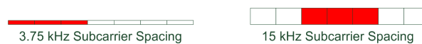
Figure 3-13: Resource elements used for demodulation reference signals in NPUSCH format 2. In this format, the RU generally occupies only one subcarrier.
