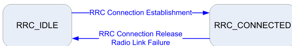
Figure 4-3: Model of the RRC states and their transitions
