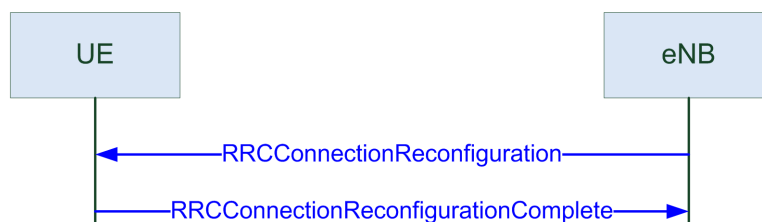
Figure 5-3: RRC connection reconfiguration procedure
