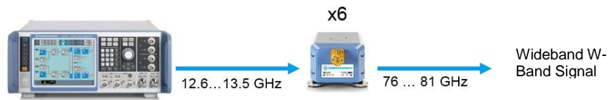
Figure 23: Simplified setup for generating wideband modulated signals at 79 GHz range, using a frequency multiplier
