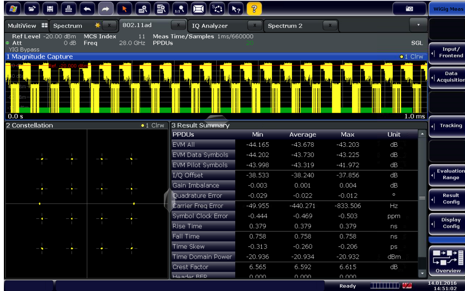
Fig. 7-1: Single Carrier signal with PAPR (Crest Factor) of 6.592 dB
