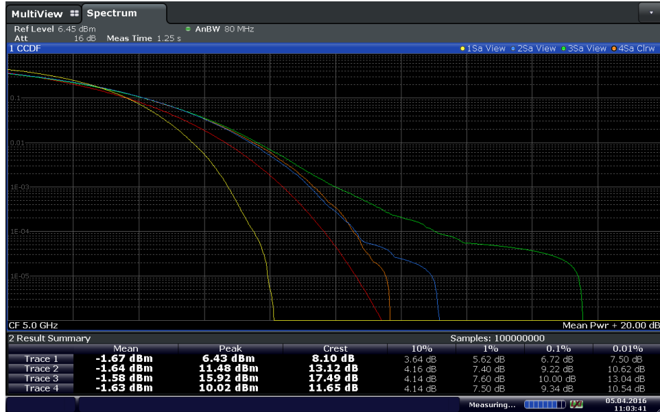
Fig. 5-7: PAPR for FBMC using different PN Sequences as payload data
