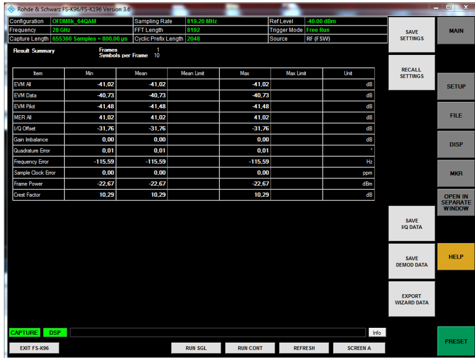
Fig. 7-2: Multi-Carrier Signal (OFDM) with PAPR (Crest Factor) of 10.29 dB
