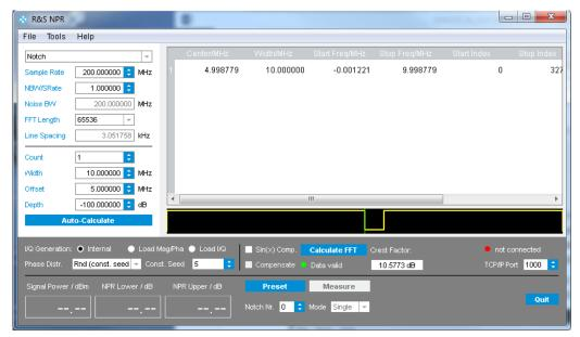
Fig. 5-44: Generate NPR test signal with R&S NPR
