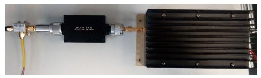
Fig. 3-11: The complete, discrete, RFFE, comprising a cascade of mixer, band pass filter and power amplifier.
