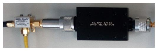
Fig. 3-9: Cascade of mixer and band pass filter
