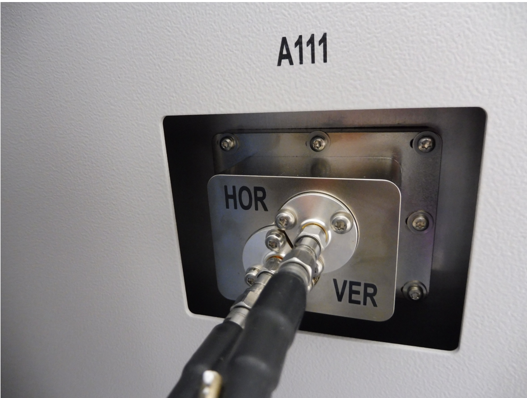
Figure 2-2: Probe antenna cables feedthrough at left face of ATS1000
