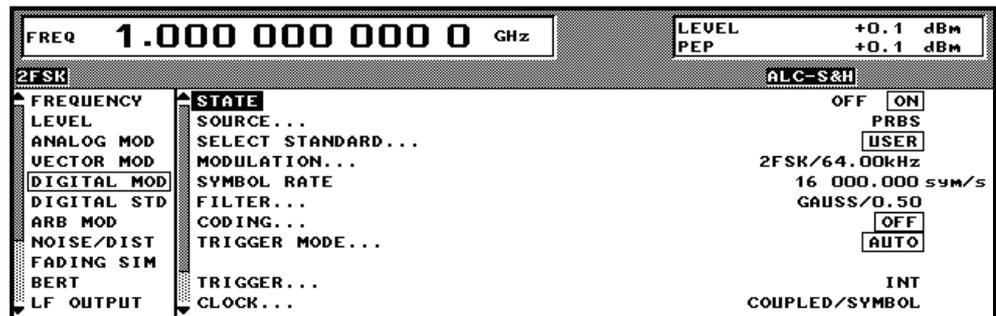
Figure 2: Modulation Setting of SMIQ
