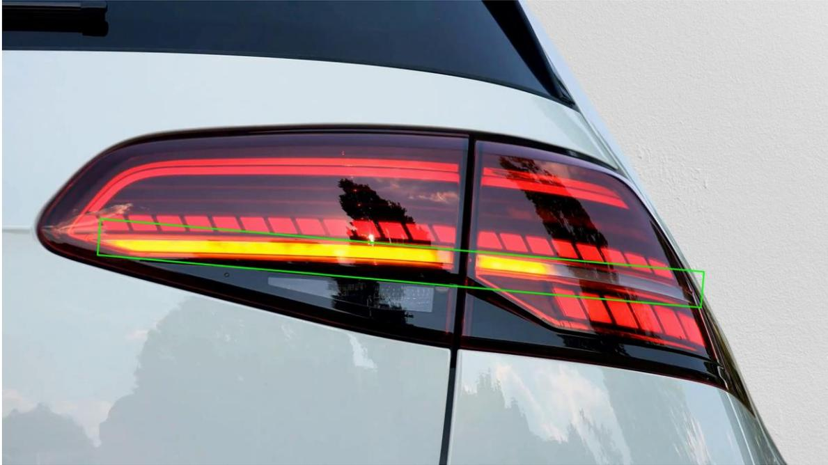
Figure 1-1: Example of a Flashing Lights ROI monitoring a dynamic turn indicator
